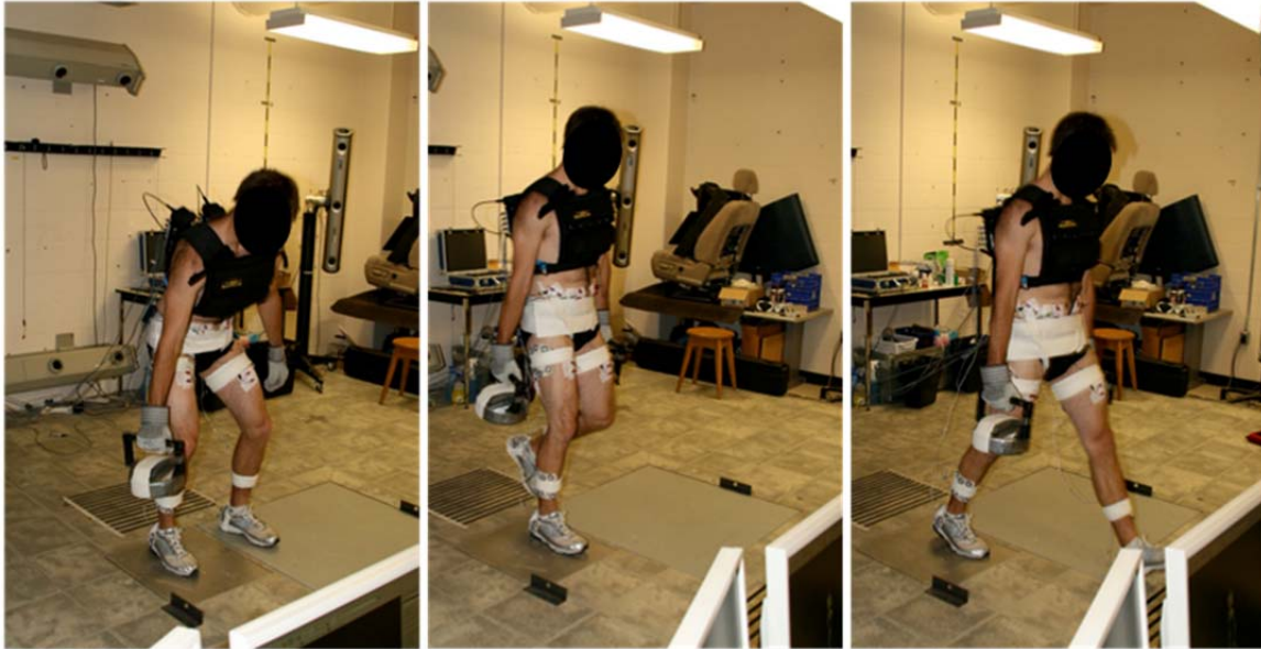
Figure 3.4. a) Equipment lift: 12.7 kg mass was lifted with the right hand from the floor; b) Equipment carry.
