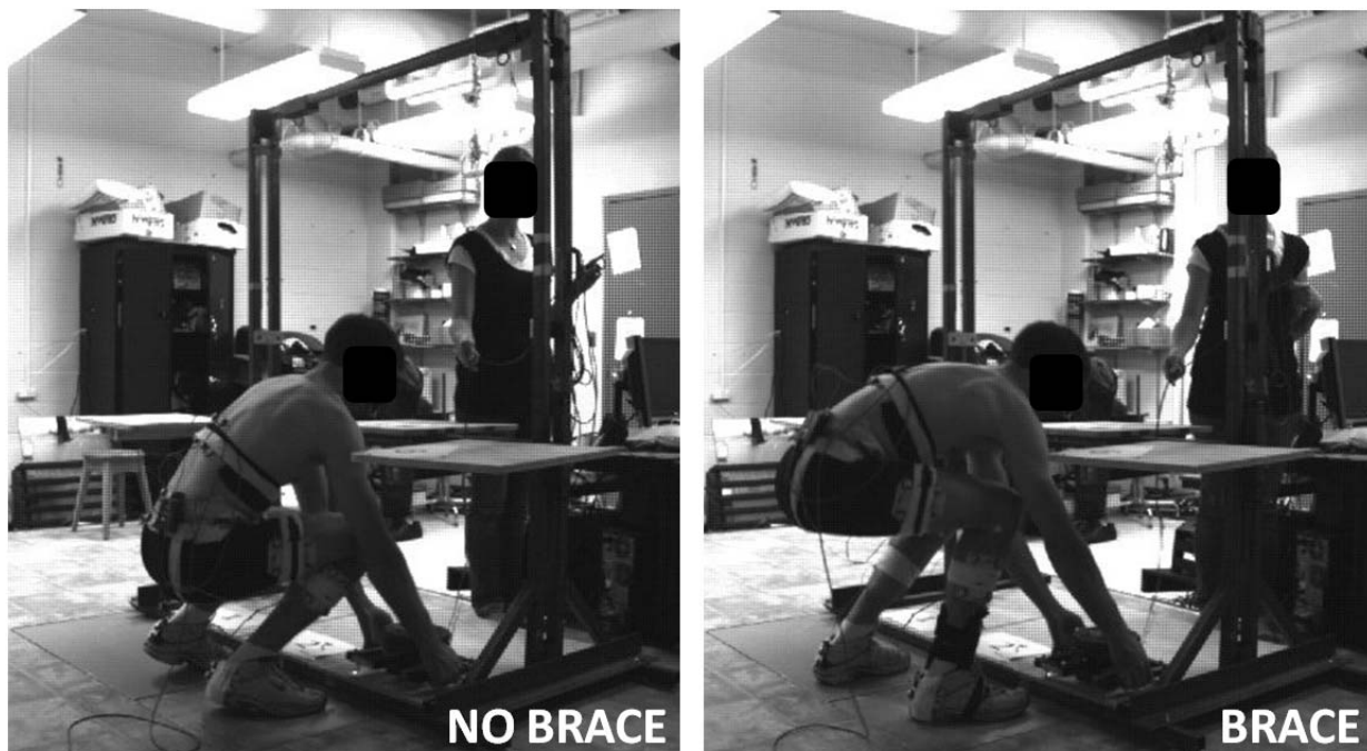
Figure 4.4. Depiction of the “group” response to unilateral ankle immobilization. When wearing the right ankle brace, subjects exhibited less ankle, less knee, greater ipsilateral hip, and greater lumbar spine motion than they did when lifting without the brace.
