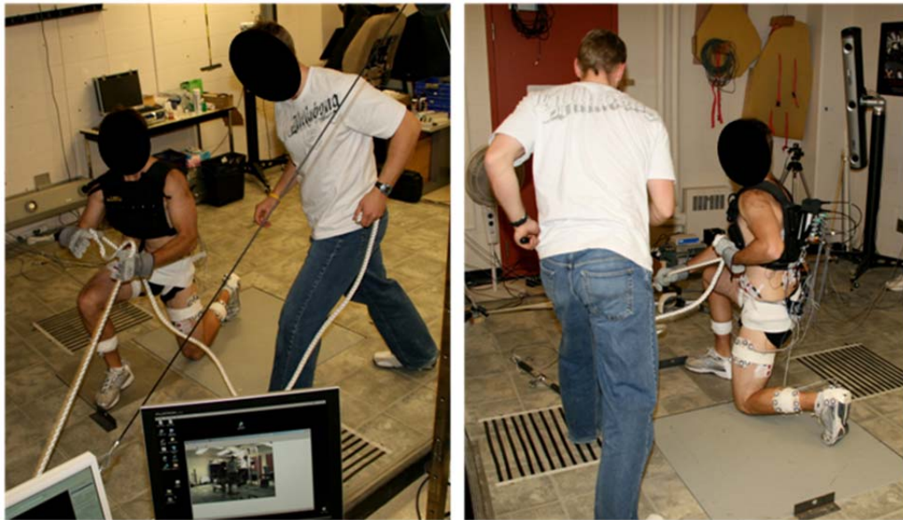
Figure 3.3. Kneeling hand-over-hand hose pull. All participants performed this task while kneeling on their left side.
