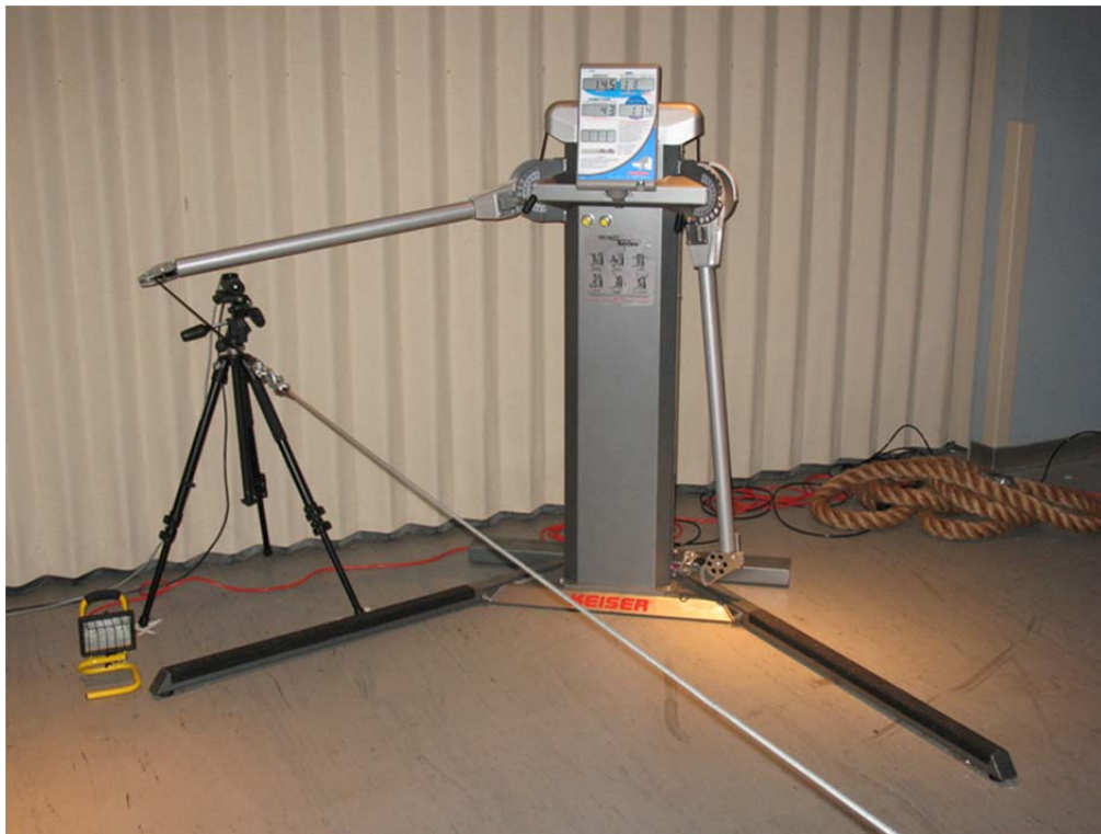
Figure 6.11. Keiser® “Functional Trainer” pneumatic cable resistance machine.
