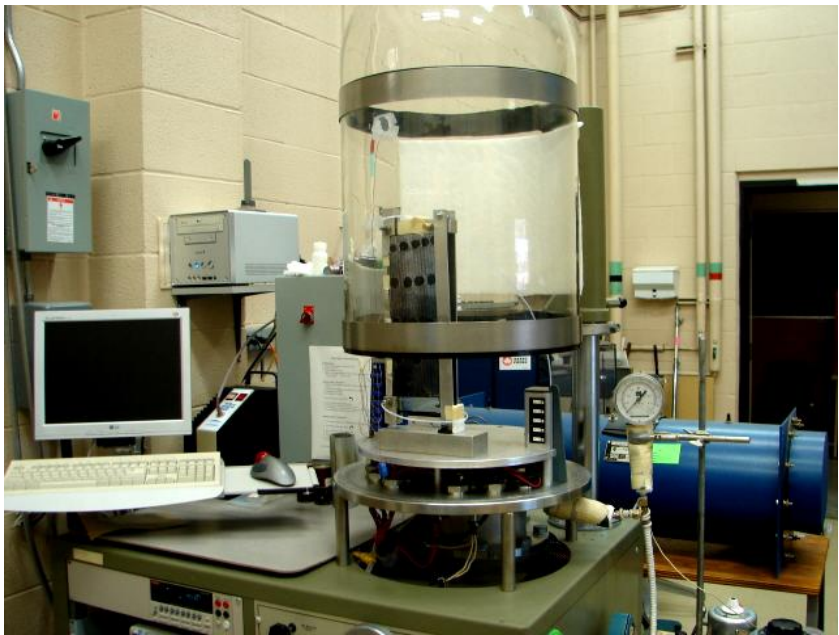
Figure 2.4: (a) Micromodel pattern geometry consisting of injector, producer, and trough, (b) A close-up of glass micromodel saturated with bitumen just before the SAGD experiment, and, (c) A snap shot of the employed vacuum test rig
