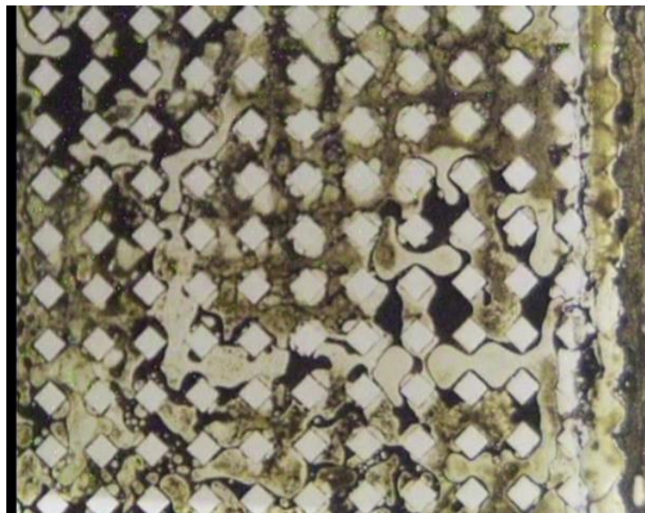
(b) Severe asphaltene precipitation within the mobilized region prevents the gravity drainage process because of the impaired vertical permeability (Run No 9: OM-1 micromodel, n-hexane as the steam additive at 15% vol/vol concentration, average operating temperature of 101.85 °C, time: 8615 seconds)
