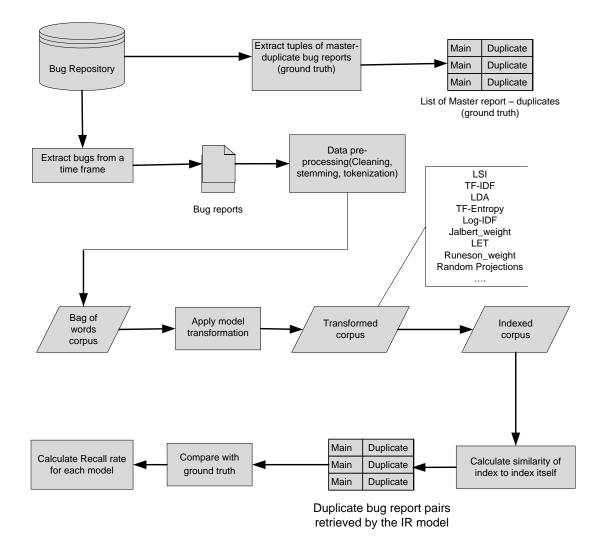
Figure 4.1: Block Diagram of Process to Determine Bug Report Similarity
