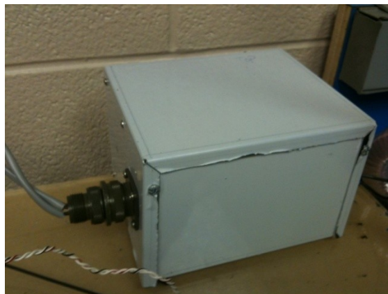
Figure 5.26. Shielding the power supply of the driver circuit in order to reduce noise.
