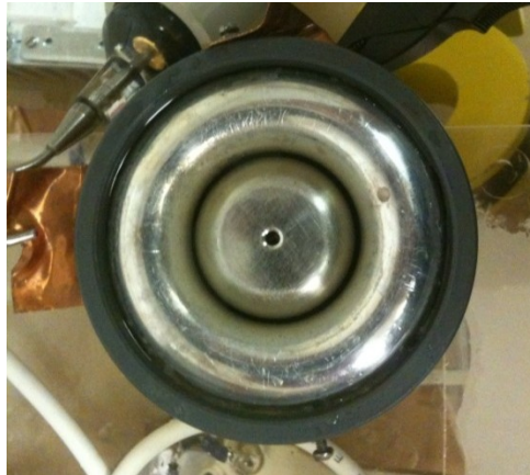
Figure 2.1. Treatment chamber showing the electrode spacing and the uniformity of the treatment zone.
