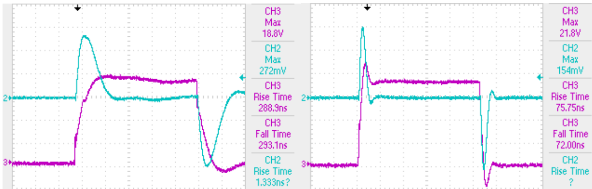
Figure 3.11. Gate voltage and current of the IXXB55N300 (left) and the CM600HA24A (right) driven by the MC4451 (12 A) chip; Voltage: CH3, 5 V/div; Current: CH2, 50 mv/A; Time 500 ns/div.
