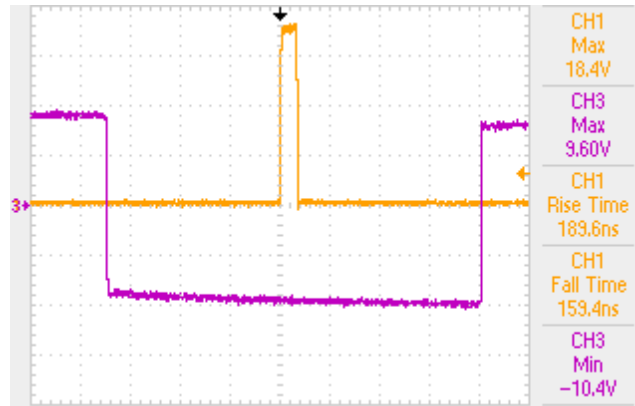
Figure 5.1. IGBT gate voltages for charging (CH1, Orange) and discharging (CH3, Purple); voltage: CH1 5 V/div; current: CH3 5 A/div; time: 10 \mu s/div.
