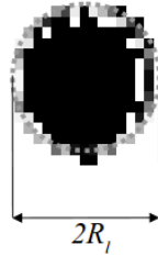
Figure 4.9: An image of the focused spot of LIFT. The gray dashed circle shows the aperture where the diameter of the spot is measured which is twice the lateral resolution of LIFT.
