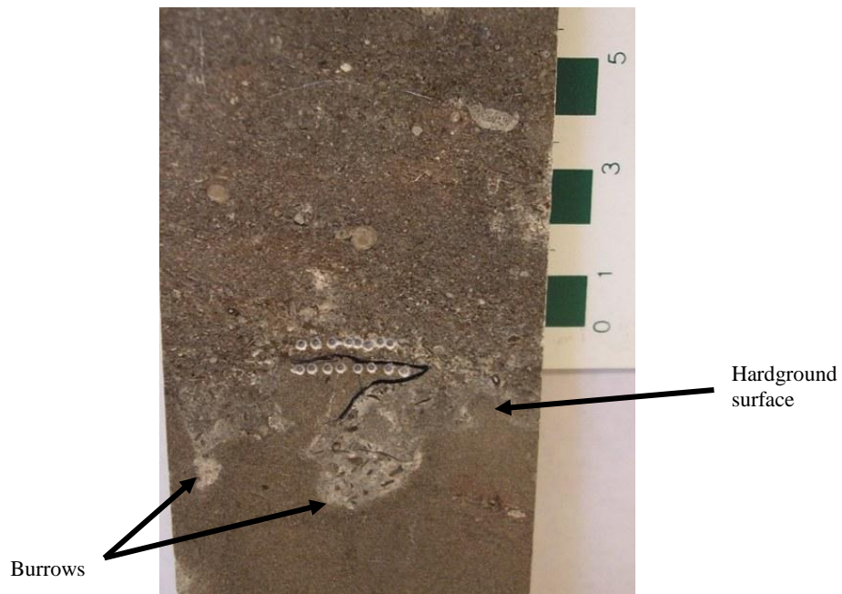
Fig. 12 Sediment is coarse-grained crinoid-rich microbioclastic grainstone. Hardground is composed of fine-grained micropeloidal bioclastic grainstone. Hardground surface is intensively burrowed (black lines highlight part of the overhang). Holes are from sample extraction for stable isotope analyses. Scale is in cm. Moore Hill Beds, Bobcaygeon Formation, OGS core 93-11-13.99.
