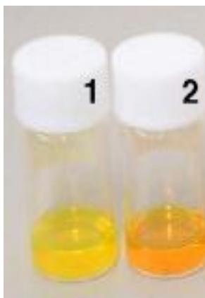
Figure 4. 1 Pictures of (a). aqueous solution of fluorescein; (b). aqueous solution of fluorescein and PDMAEMA- C_{60} .
