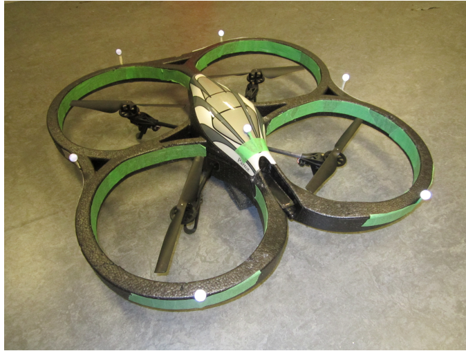
Figure 5.1: AR.Drone Parrot quadrotor.
