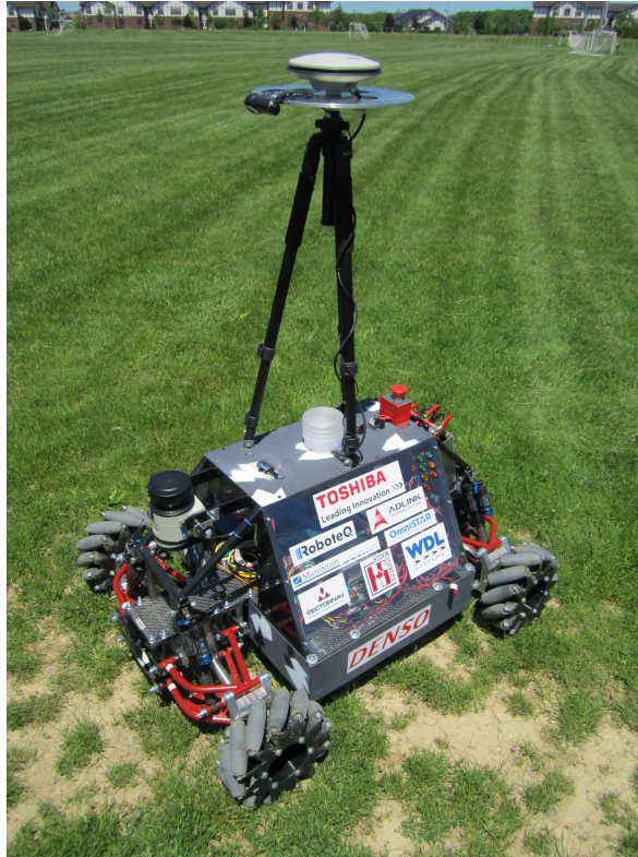
Figure 5.5: Custom built skid-steer UGV (University of Waterloo’s 2011 IGVC entry).
