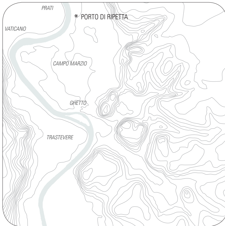
fig. 1.96 The Tiber River at its normal water level around 5 masl. Shown with the topography lines (at 5m intervals) of the pre-embanked river condition in Rome. Today, Rome's elevation ranges from 13 masl at the Pantheon to 139 masl at the peak of Monte Mario. (Chelys 2008)
