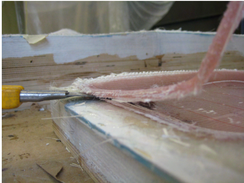
Figure A.15: Green trimming - detail.
