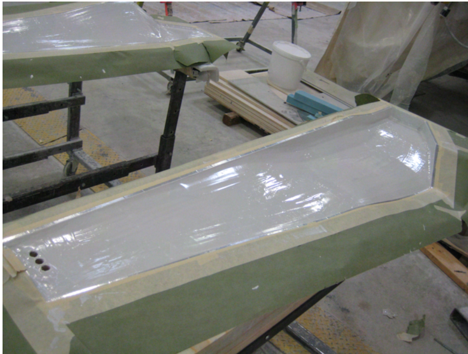
Figure A.9: Gel coat applied to entire mold.
