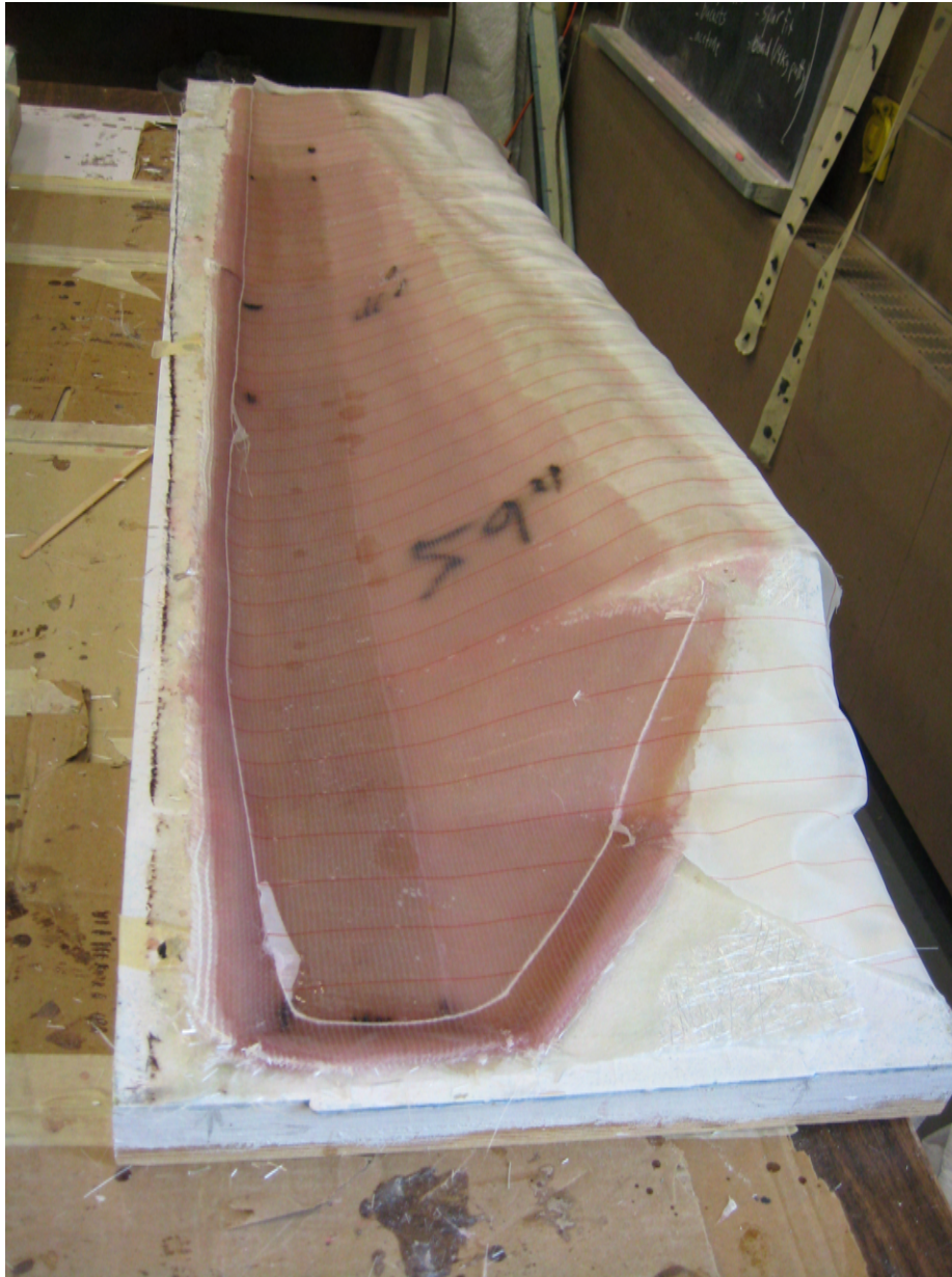
Figure A.12: Mold with structural layers and peel-ply.
