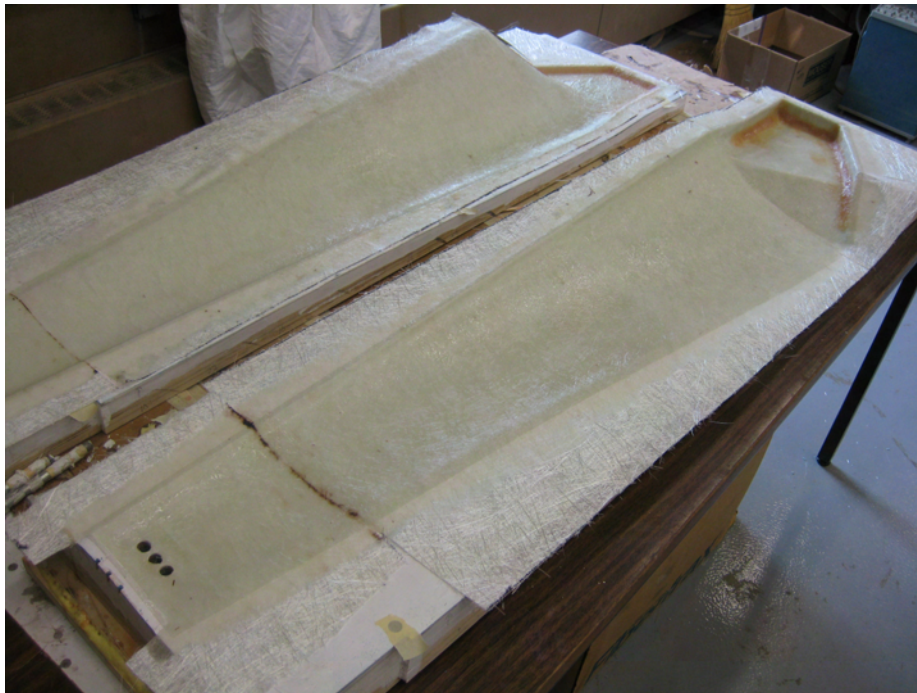
Figure A.10: Mold with skin layer applied.
