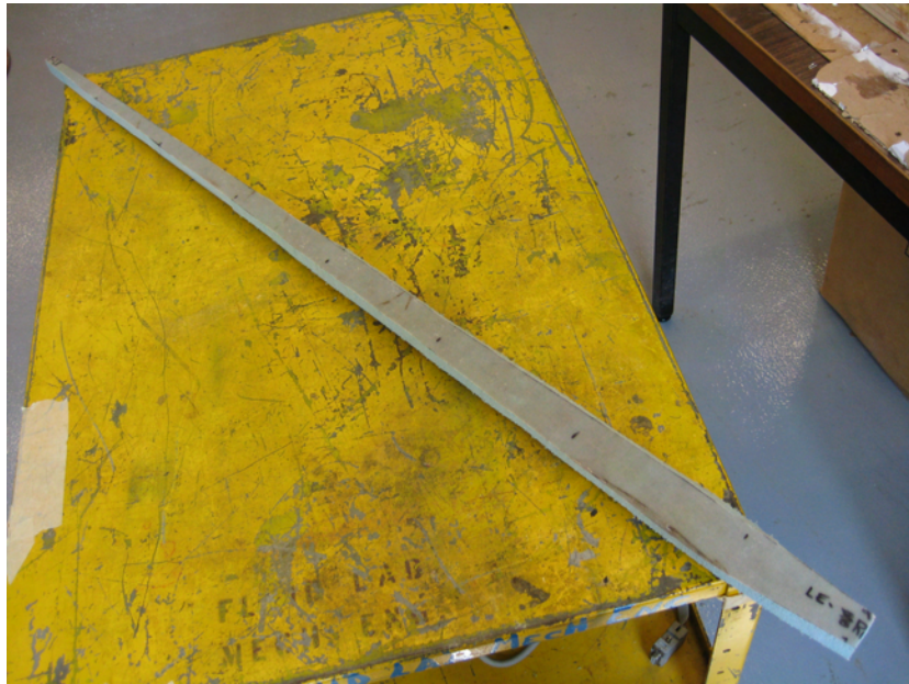
Figure A.18: Spar cut to inner dimensions of blade.
