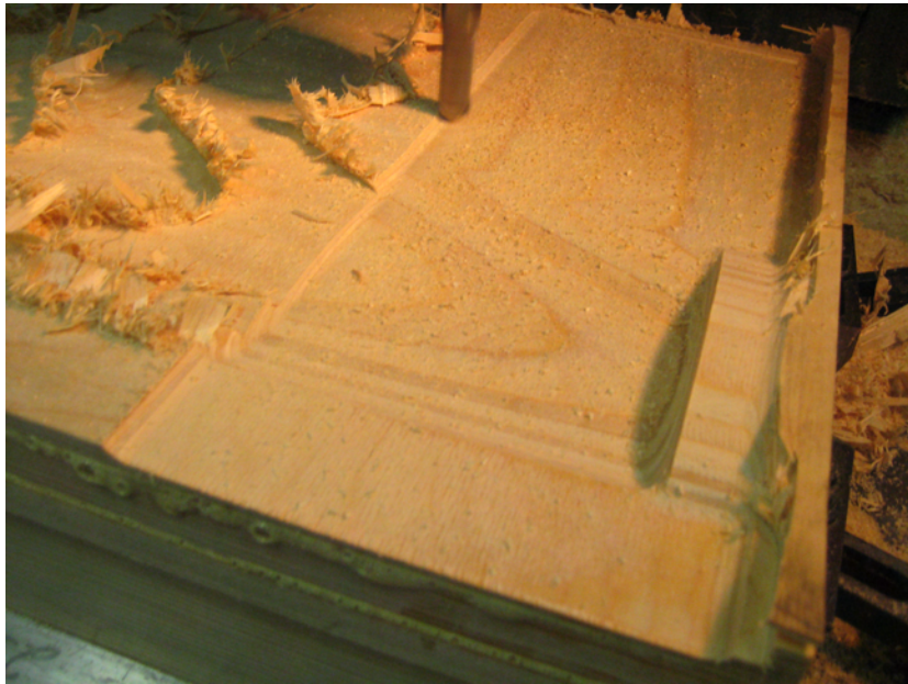
Figure A.4: Milling the mold.
