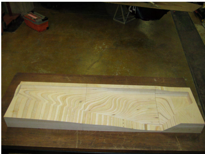
Figure A.5: Mold upon completion of milling.
