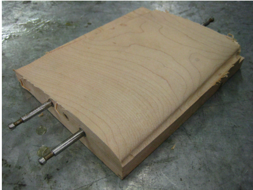
Figure B.5: Tip in between having first and second surface milled.
