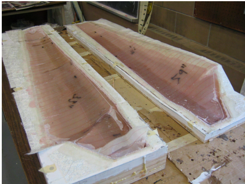
Figure A.16: After green trimming.
