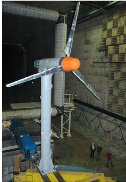
Figure 2.21: MEXICO turbine mounted in DNW LLF wind tunnel. From Schreck et al. [32].
