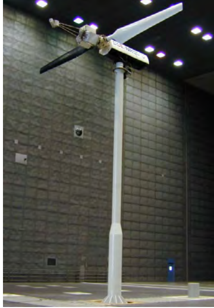
Figure 2.16: UAE Phase VI turbine mounted in NASA Ames 24.4 m x 36.6 m wind tunnel. From Schreck et al. [32]).
