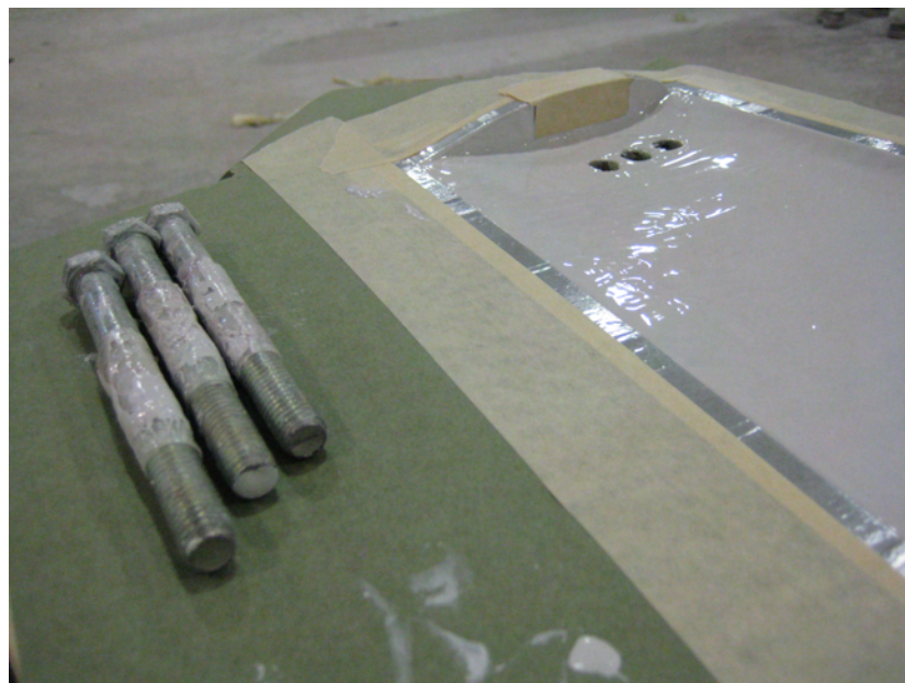
Figure A.8: Gel coat applied - bolts and tape removed.
