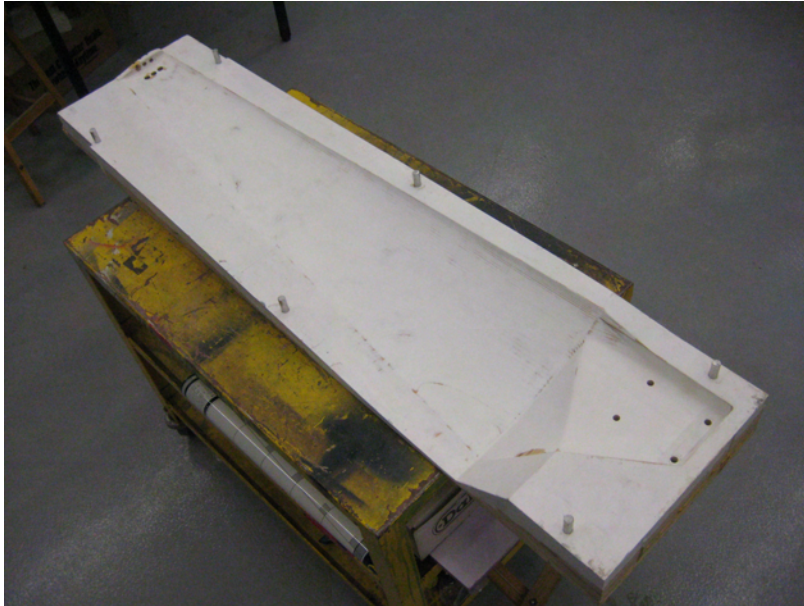
Figure A.6: Finished suction side mold with alignment dowels inserted.
