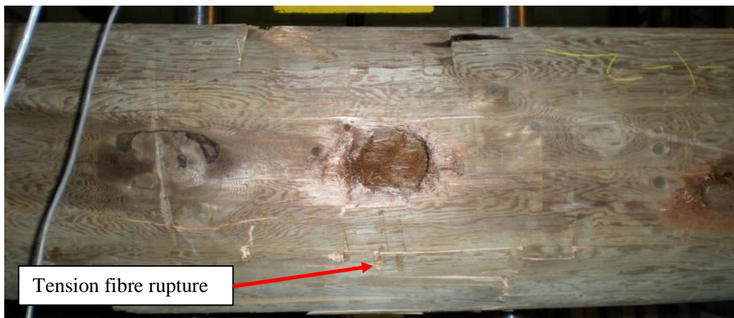
Figure 89. - Tension fibre rupture of in-service specimen with neutral axis damage (C-1-2).
