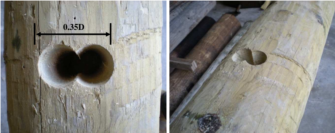
Figure 19. - New pole specimen idealized nesting damage.
