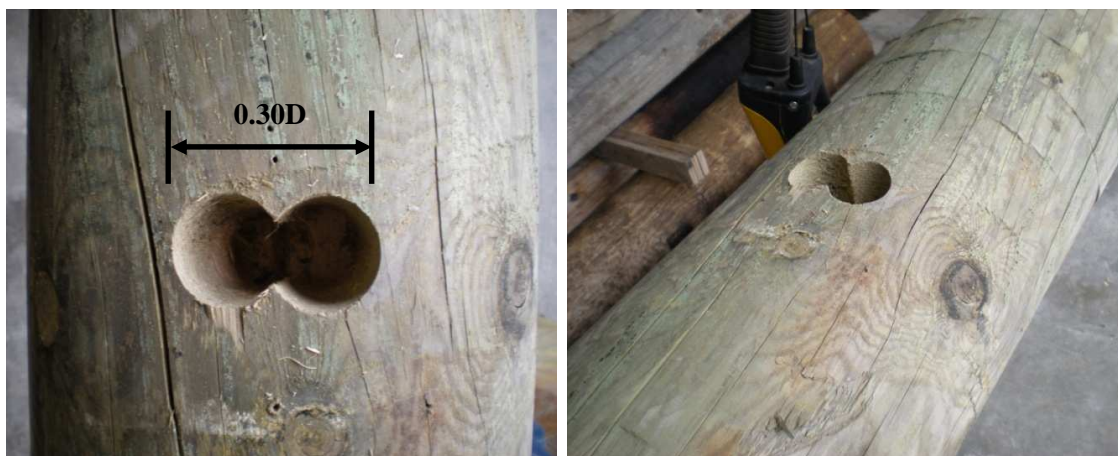
Figure 18. - New pole specimen idealized feeding damage.
