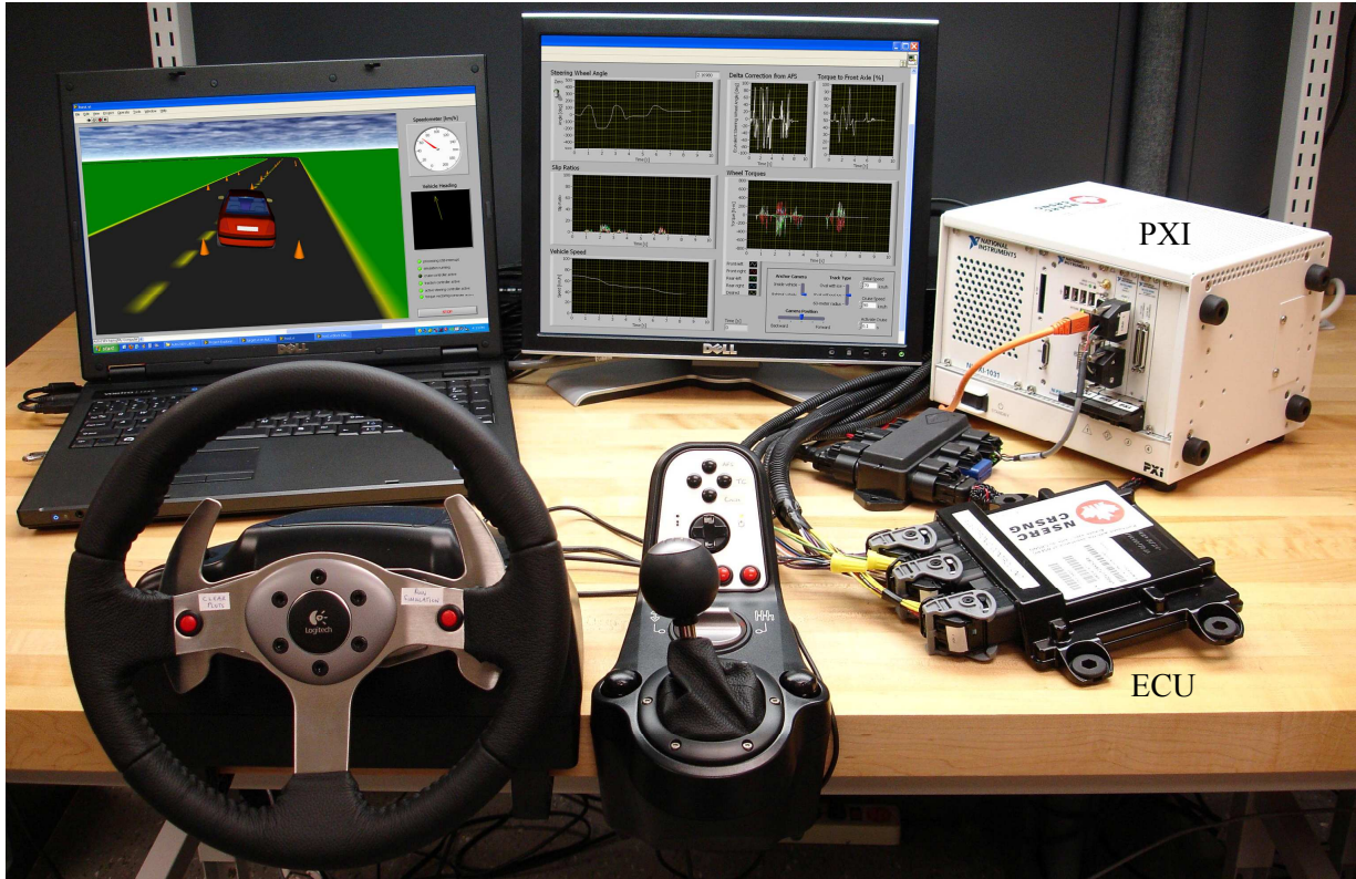
Figure 6.1: Hardware- and operator-in-the-loop driving simulator
