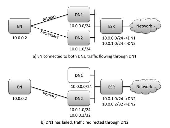
Figure 3.2: System Prior to (a) and Following (b) Failure of a DN
