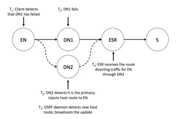
Figure 3.5: Timeline Of System States During Failover
