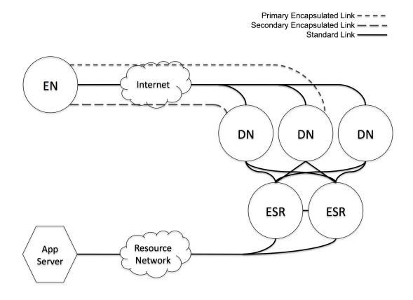
Figure 3.1: Failover Encapsulation Architecture
