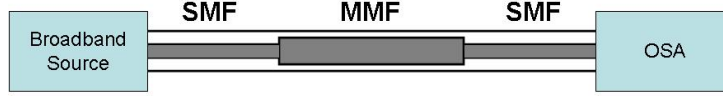
Figure 2.11: Schematic of all-fiber multimode fiber interferometer. SMF: single-mode fiber; MMF: multimode fiber; OSA: optical spectrum analyzer.
