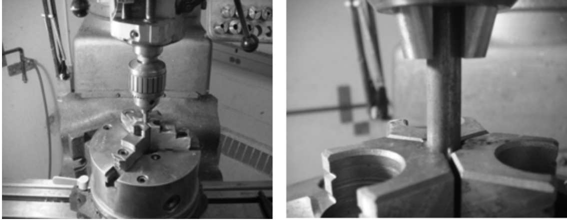
Figure 3.7: Center the tool holder on the steel rod.
