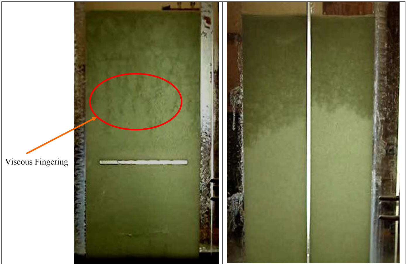
Figure 4.36: Schematic of viscous fingering phenomenon in the fractured porous medium[ b= 5 \text{ mm} , fluid pair=CMC solution (2%)-Air , BT3 glass beads , q = 1.4 \text{ cm}^3/\text{s} ]
