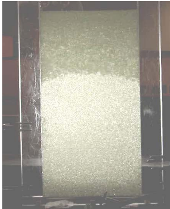
Figure 4.7: Snap shot of G-L interface advancement [matrix filled with BT2 glass beads, Fluid pairs: Air-CMC solution (1%), b = 5 mm, Model height = 55 cm, liquid pumping rate: 1.8 \text{ cm}^3/\text{s} ].
