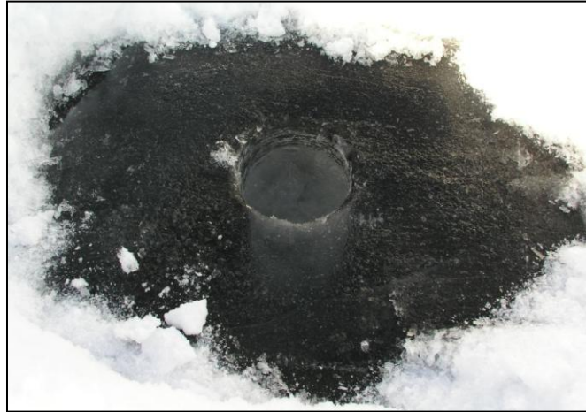
Figure 2-1: Congelation/Black Ice in Inuvik, NWT. Note that the drill hole can be seen through the clear ice. Source: Toose, P., Inuvik Field Campaign, (2008).
