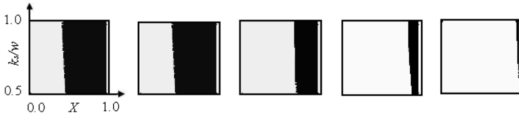
Figure 3.10: Applicability of GA model with variable dimensionless water table depth (Left to right: 1/40, 1/30, 1/20, 1/10, and 1/5 ): Light-applicable; Dark-non-applicable
