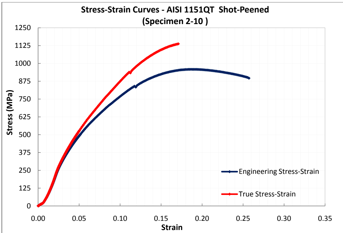
Figure 4.6. Engineering and true stress-strain curve for shot-peened AISI 1151QT
