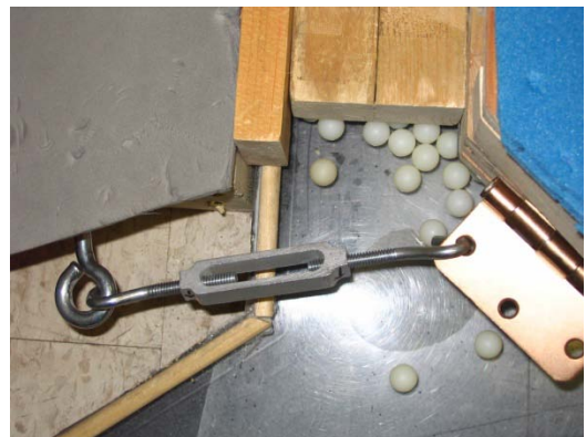
Figure 8-3: Close-up view of the turnbuckle and bolt/hinge system used to secure the upper and mid-sections of the frictionless jig.
