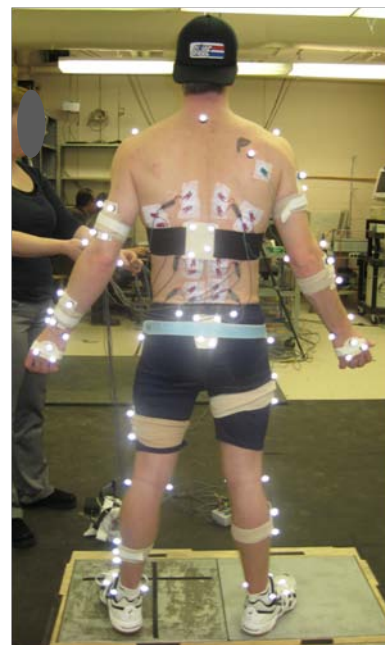
Figure 5-1: Posterior view of participant with reflective markers and EMG electrodes in place.
