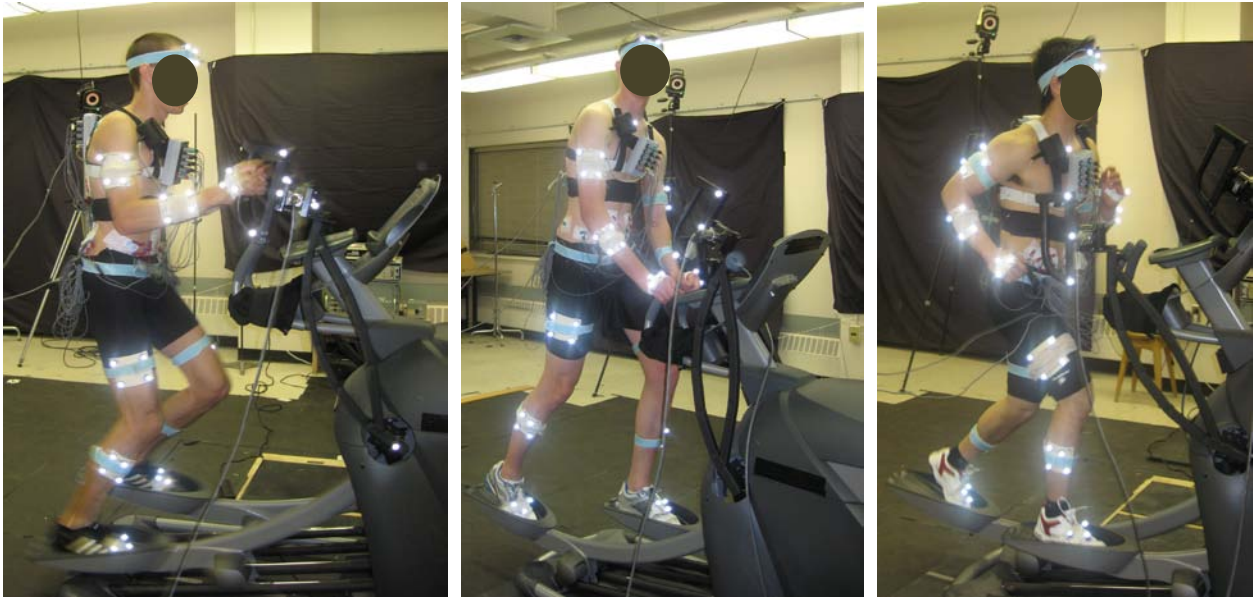
Figure 9-2: Photographs of participants on the elliptical trainer in the three positions tested. Left to right, they include: hands holding onto the handles, holding onto a central bar, and free-hand.
