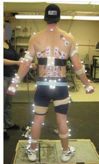
Figure 9-1: Posterior view of participant with reflective markers and EMG electrodes in place.
