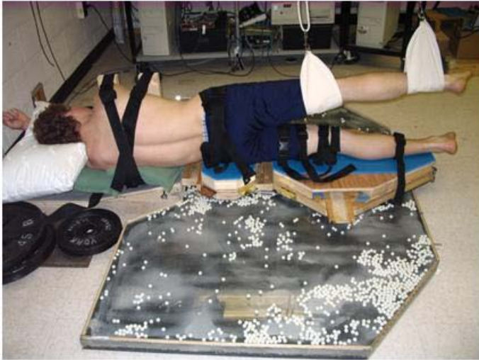
Figure 8-2: Position of participant on the frictionless jig. In this specific scenario, the right leg is suspended from the ceiling, allowing free movement of the left hip.
