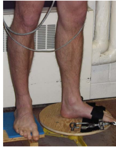
Figure 7-4: Left hip ER, illustrating the eye-bolts and carabineer in series with the force transducer.
