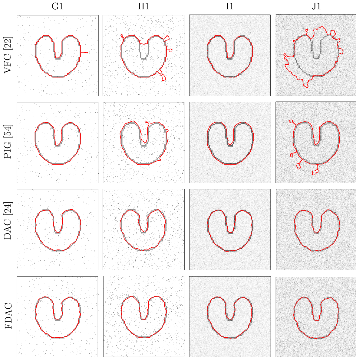
Fig. 5.11: The noise robustness of FDAC compared to PIG [54], VFC [22] and DAC [24] on a synthetic u-shape object. The four noisy images are generated by adding gaussian noise of variances 0.01 and 0.1 and salt and pepper noise of variances 0.01 and 0.03. Rows and columns present images and methods. FDAC and DAC successfully identified the true boundary for all noisy images. PIG successfully identified the boundary of all images except J1.
