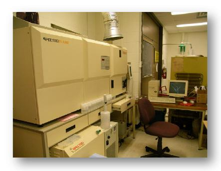
Figure 3-10 ICP-AES used for sulfur species analysis
