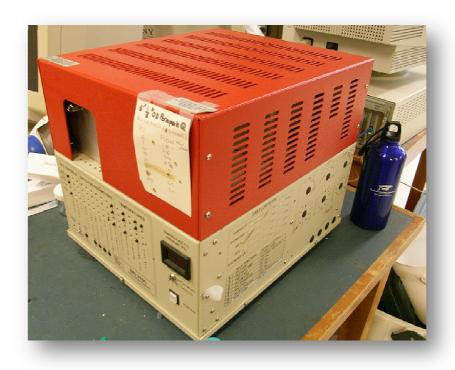
Figure 3-6 GC-TCD for methane and carbon dioxide analysis
