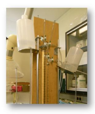
Figure 3-5 Manometer device for gas volume measurement
