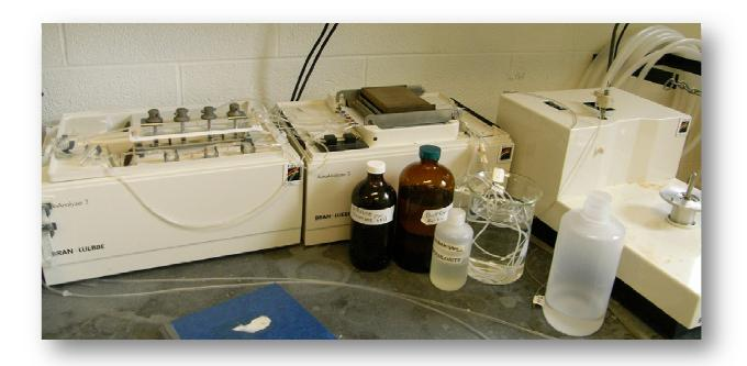
Figure 3-4 Automatic ammonia analyzer
