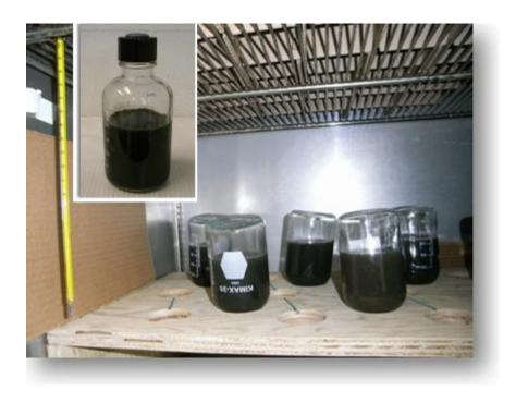
Figure 3-2 Serum bottle and their set-up in the isothermal incubator
