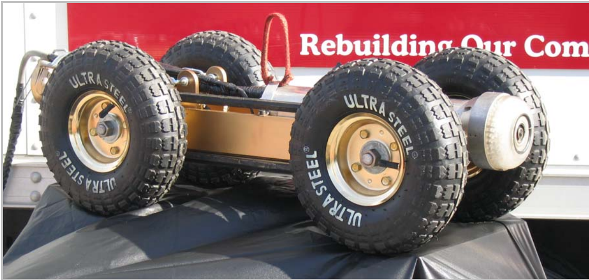
Figure 3.3: PipeFlo Contracting Corp. and the City of Niagara Falls Owned SSET Camera
