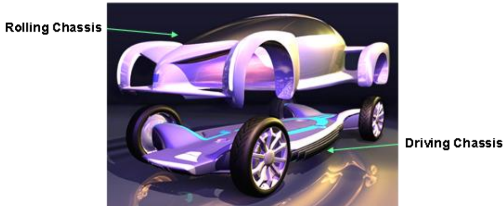
Figure 1-2: GM Hy-wire concept car with rolling and driving chassis [Elb04]
