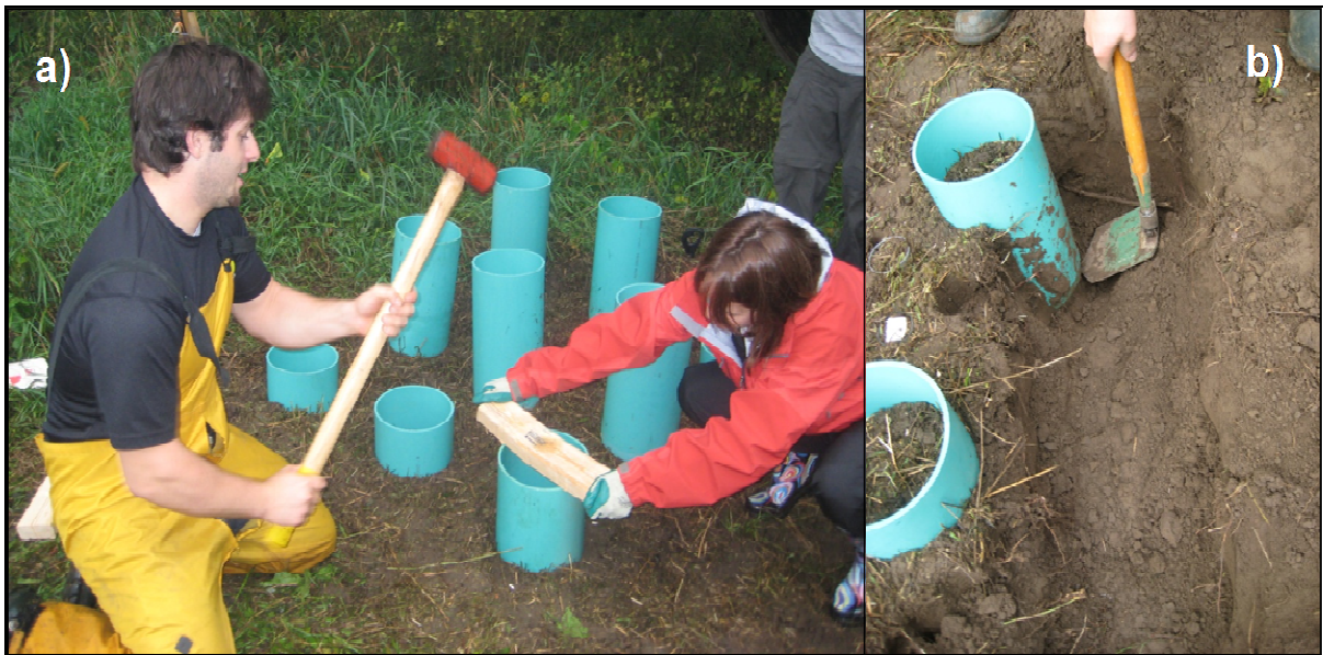
Figure 4- Photos showing insertion of monolith casings into soil (a) and monolith removal (b).
