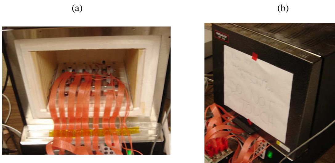
Fig. 32 (a) Chips fastened to the rig and placed in oven. (b) Oven door closed over cabling.
