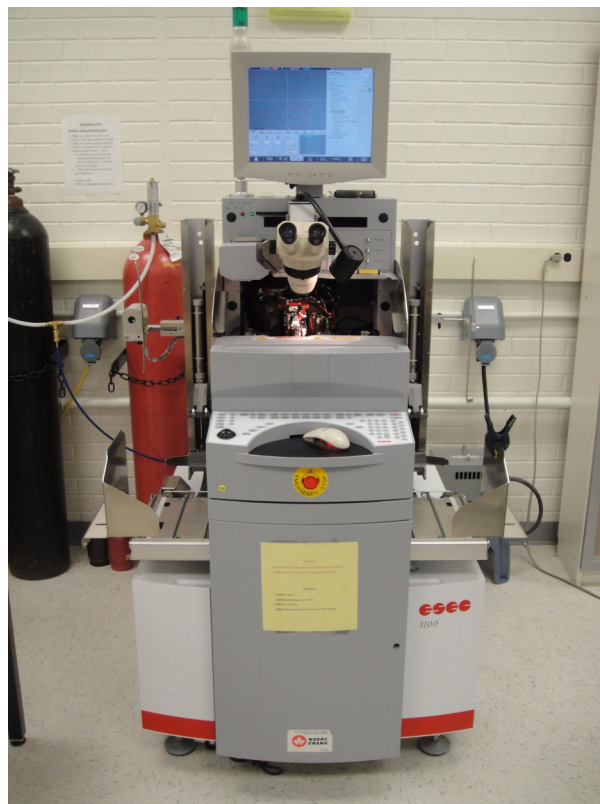
Figure 17: Besi Esec 3100 automated thermosonic wire bonder.
