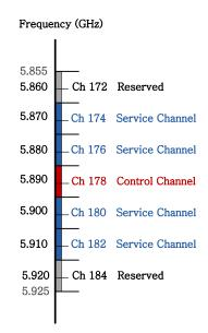
Figure 2.3: DSRC spectrum allocation by FCC.
