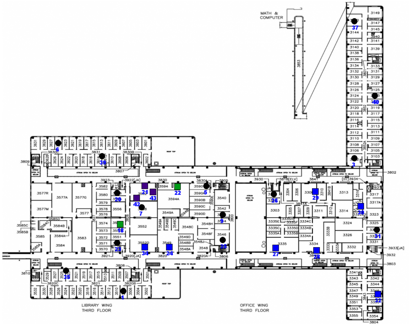
Figure 4.1: WLAN testbed on the 3rd floor (circles represent clients and squares represent APs. However, this is just annotation and the actual configuration can be changed by the person configuring the testbed)
