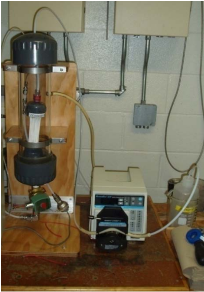
Figure 3-7 View of the holding tank and the hollow fiber UF membrane
