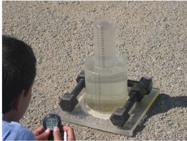
Figure 4-2 Apparatus Set-Up for Permeability Test on PCPs.
