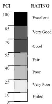
Figure 2-2 Pavement Condition Index and Rating Scale (ASTM D 6433 2007).
