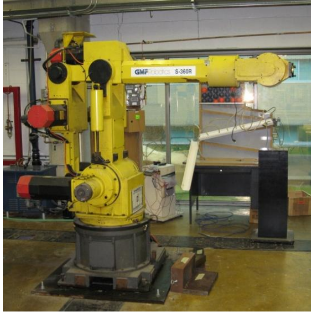
Figure 2.5: Fanuc S-360 Industrial Manipulator
