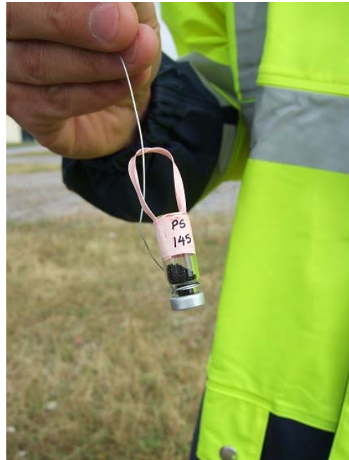
Figure 6-2: Photograph showing supports for sampler installation.
