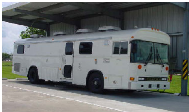
Figure 6-6: US EPA TAGA mobile laboratory
