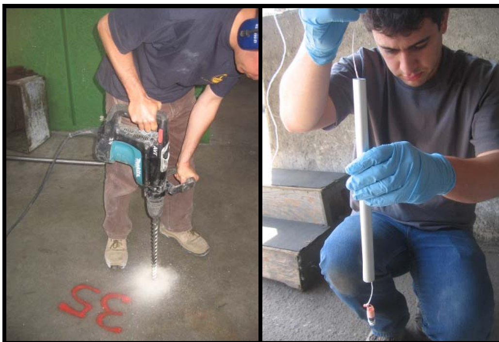
Figure 7-8: Photographs of (A) – a hole being drilled into the floor and (B) – deployment of the TWA-PDMS sampler at a predetermined depth in the hole.
