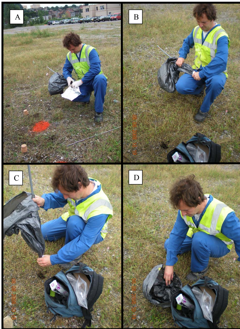
Figure 7-2: Photographs of (A) – Aluminum foil being wrapped around the plastic cover, (B) – crunching the aluminum foil for snug fit, (C) – the assembly being inserted into the borehole and (D) – the completed borehole sealing process.
