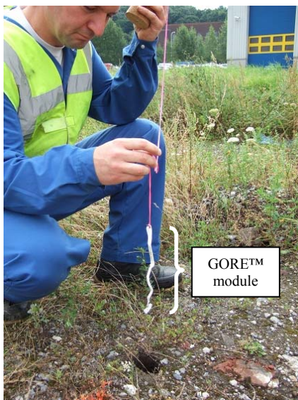
Figure 7-3: Deployment of the GORE™ module inside a borehole.
