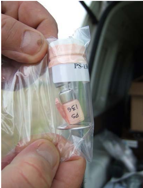
Figure 6-1: Photograph of a TWA-PDMS sampler packed and shipped to the field.
