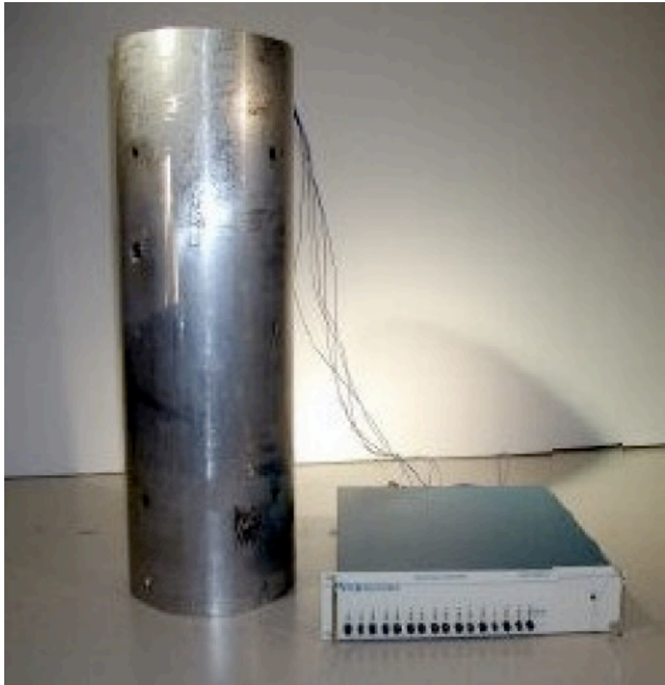
Figure 27: An instrumented Blast Test Device [CHPPM, 2005]
