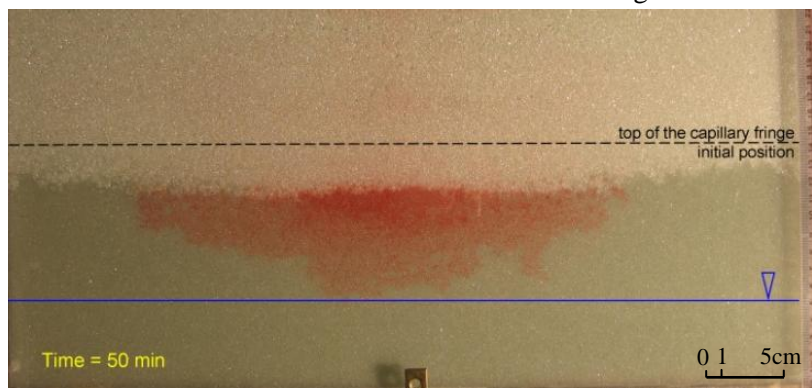
b) Later times: gasoline spreading is preceded by capillary fringe collapse
