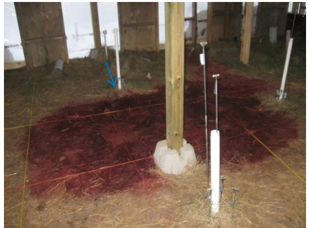
Jan. 22 nd , 2009 (day 154) – WT = 36cm bgs: Red stain is stronger and covers a bigger area. Stain is also seen outside of the temporary building. Blue arrow shows groundwater flow direction.
