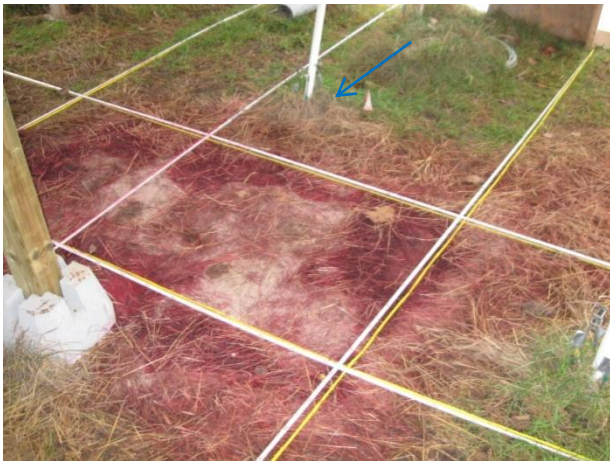
Dec. 03 rd , 2008 (day 104) – WT = 41cm bgs: Red stain is stronger on the sides of the trench. Gasoline likely accumulated more on these regions due to less effective packing on the sides. Blue arrow shows groundwater flow direction.
