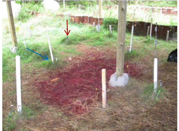
Sep. 17 th , 2008 (day 27) – WT = 49cm bgs: Red stain on the ground after water table rise. Blue arrow shows groundwater flow direction. Gasoline was recovered at the vapor sampling port indicated by the red arrow at 40 and 60cm bgs.
