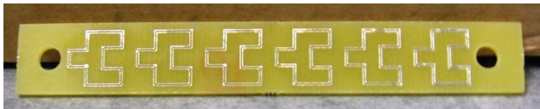
Figure 4.4: A single strip containing 6 unit cells of inclusions fabricated using printed circuit board technology.
