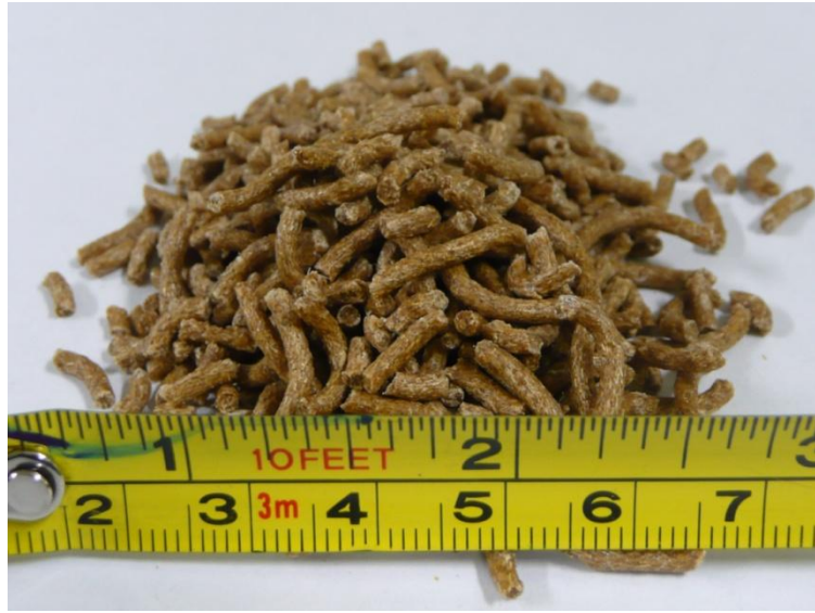
Figure 3-2 WSCPP Pellets Obtained From Compounding Process by Minilab
