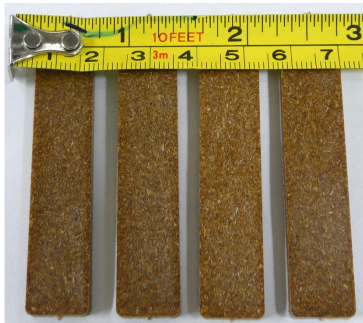
Figure 3-3 WSCPP Test Sample Bars Obtained From Injection Molding Process
