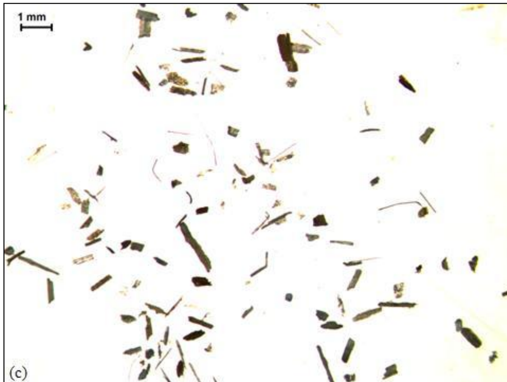
Figure 4-6 Wheat Straw Particles in Fraction 60-100 (a) Large (b) Mid size (c) Fine
