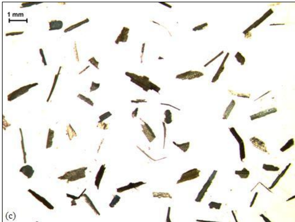
Figure 4-5 Wheat Straw Particles in Fraction 35-60 (a) Large (b) Mid size (c) Fine
