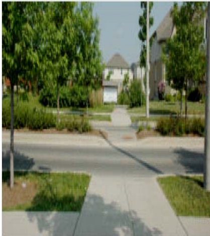
Figure 34, Barrier Free Median
