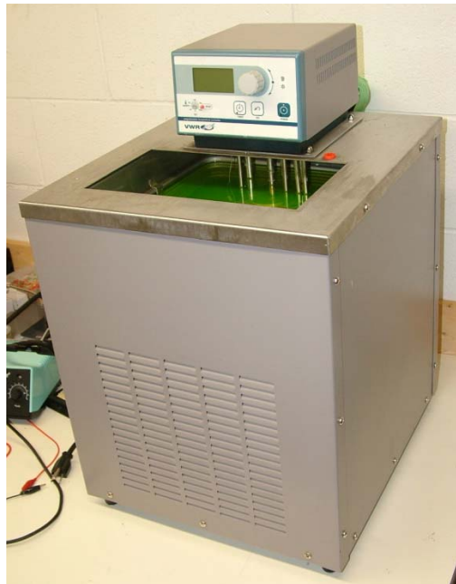
Figure 7-3 VWR refrigerating circulator with programmable temperature controller
