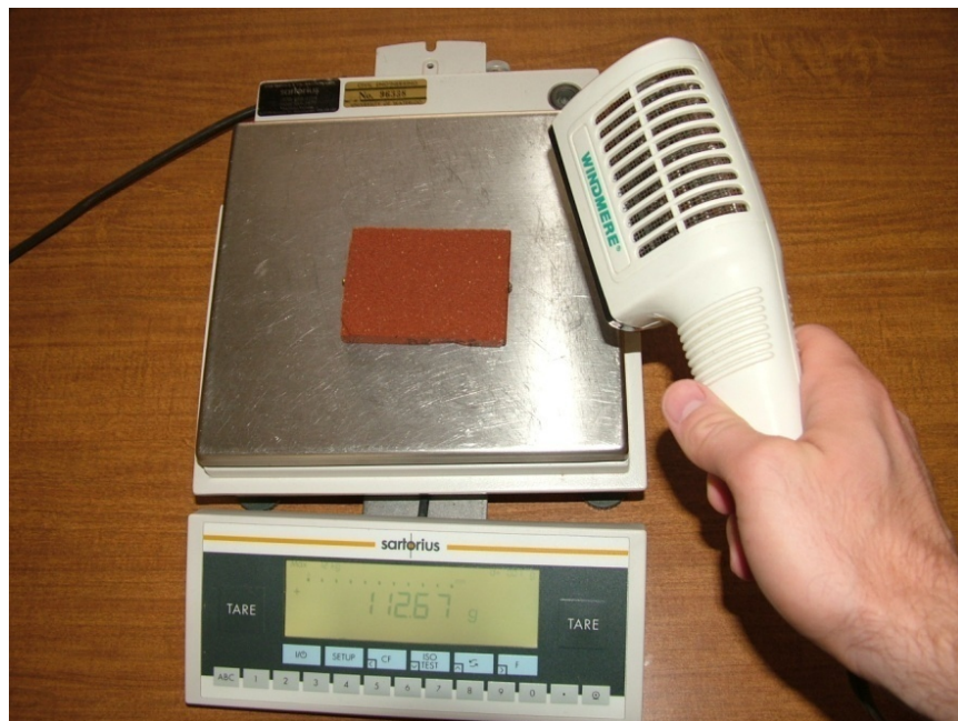
Figure 6-2 Drying a saturated specimen to a target moisture content
