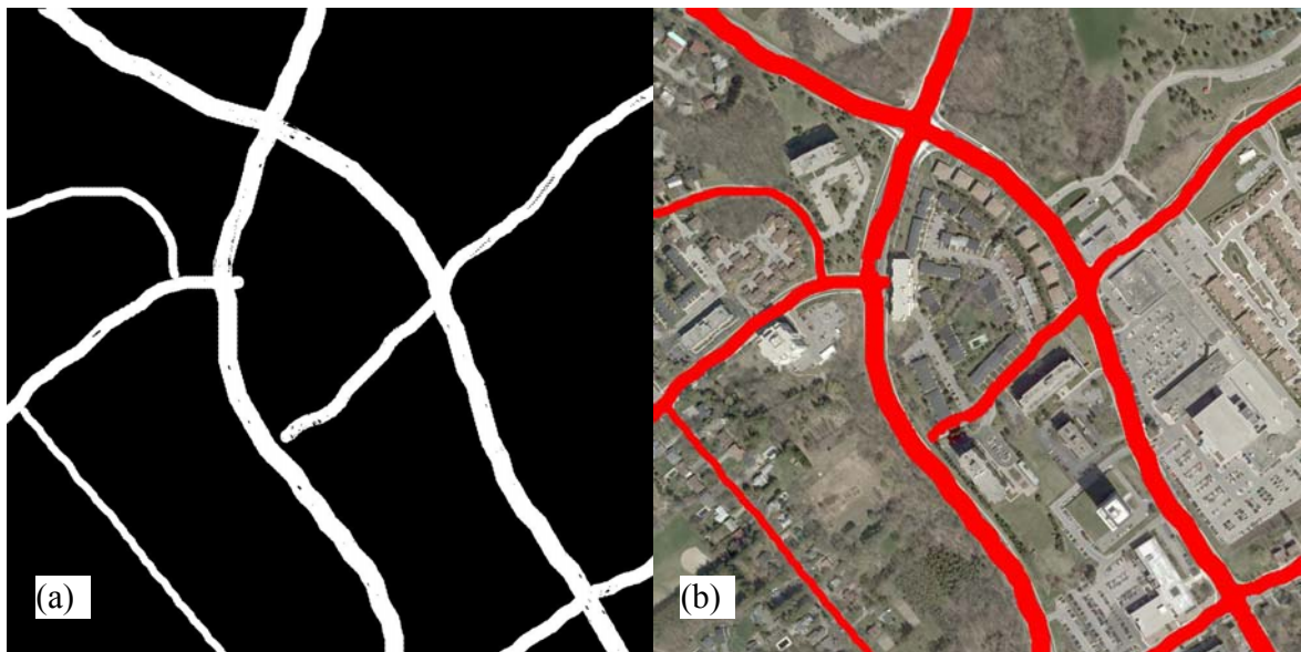
Figure 4.11 Morphologically filtered roads with shadows and overlaid on the image
