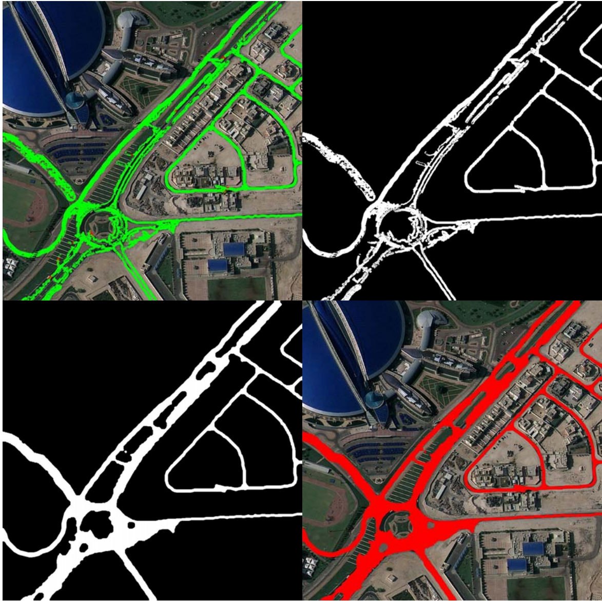
Figure 4.8 Morphologically filtered roads with roundabouts and overlaid on the image
