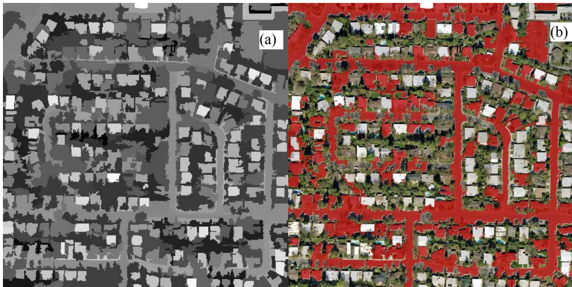
Figure 4.18 Roads with numerous trees detected by the object-oriented classification
