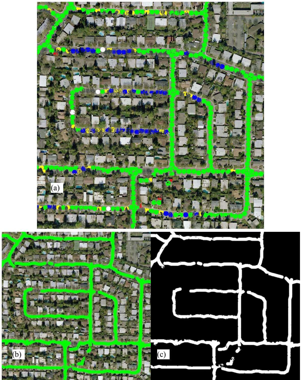
Figure 4.19 Roads with numerous trees detected by the RoadModeler
