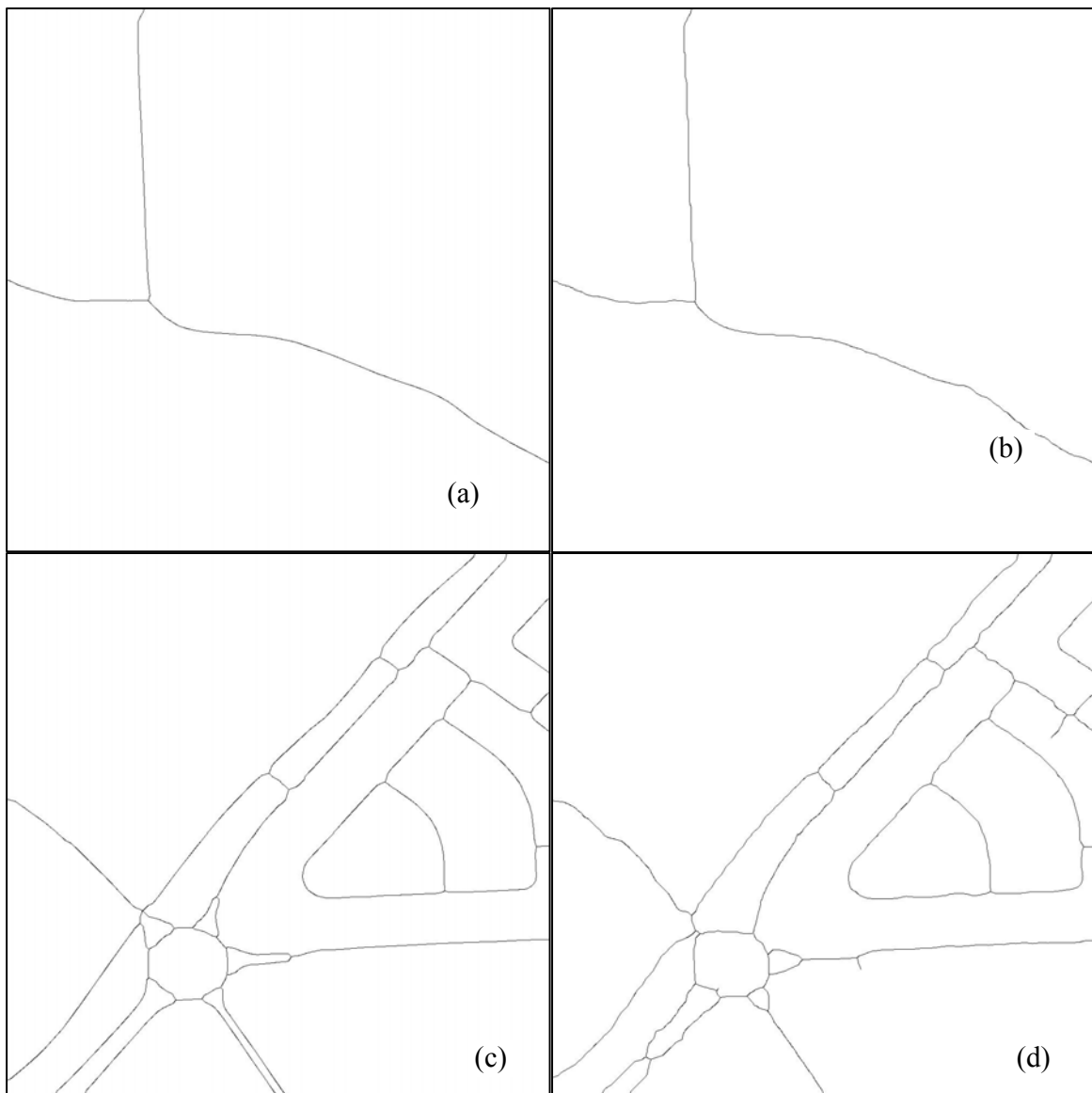
Figure 5.2 Reference vs. extracted road centerlines of GeoEye-1 satellite images: (a) and (c) Reference centerlines generated by on-screen manual digitizing, (b) and (d) centrelines extracted by the RoadModeler
