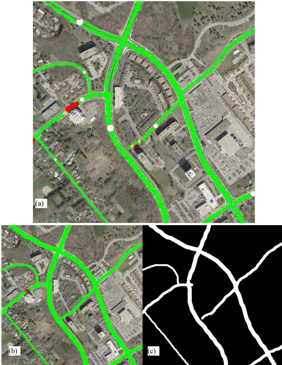
Figure 4.10 Roads with shadows detected by the RoadModeler
