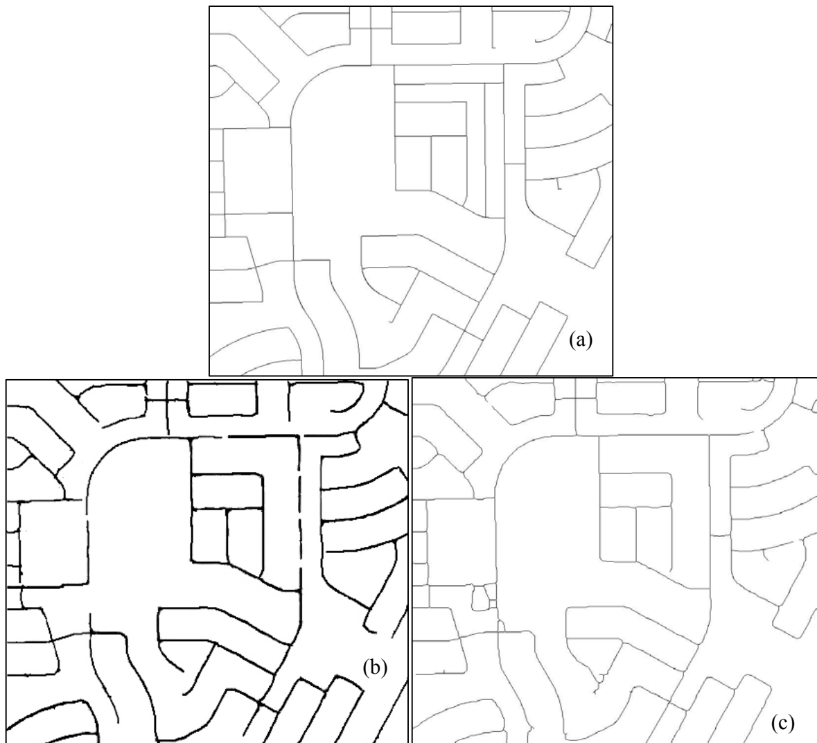
Figure 5.5 Reference vs. extracted road centerlines of black and white aerial image: (a) Reference centerlines, (b) centerlines extracted by Hu et al (2007), (c) centerlines extracted by the RoadModeler
