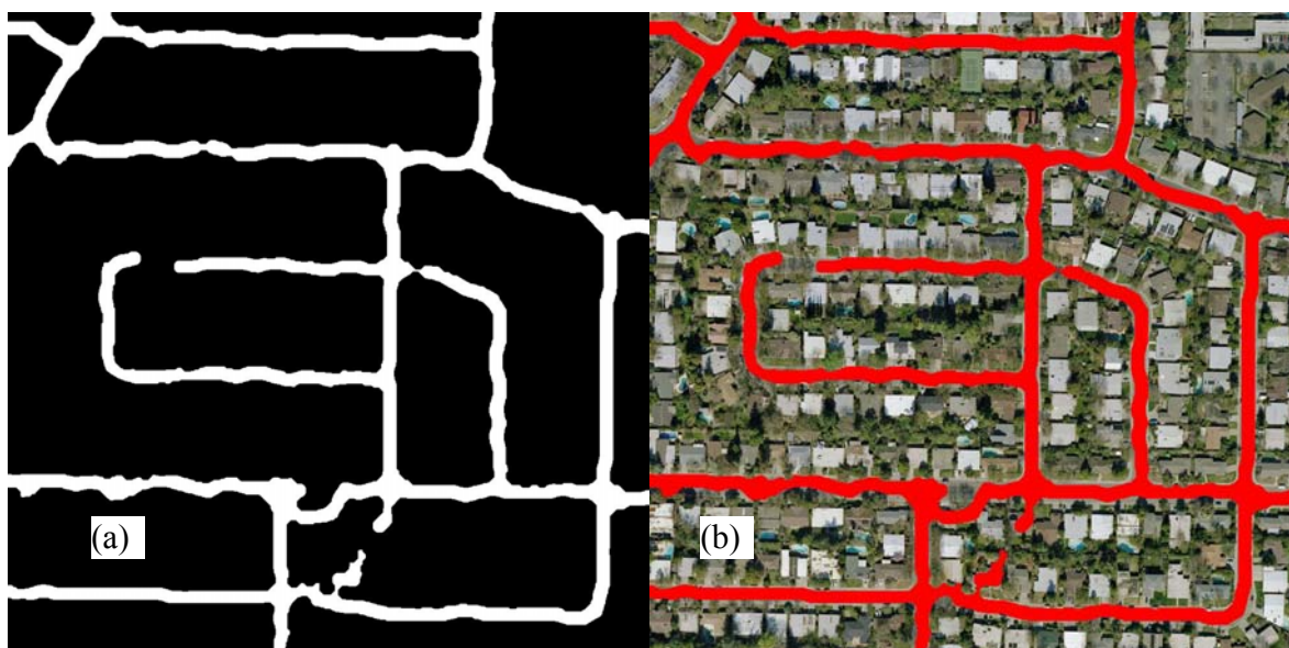
Figure 4.20 Morphologically filtered roads with numerous trees and overlaid on the image
