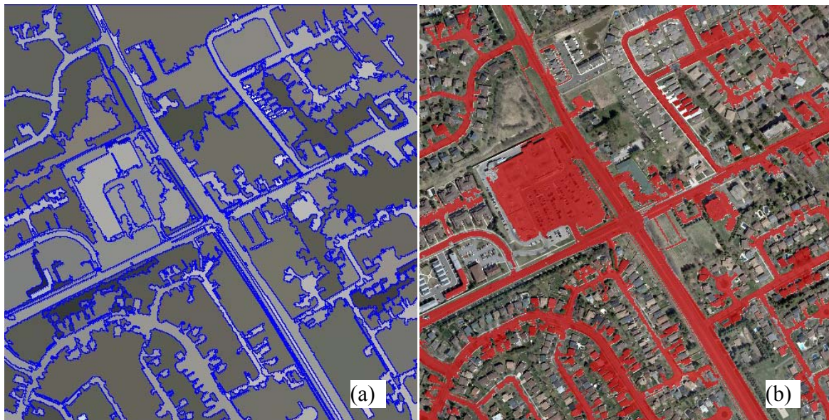
Figure 4.12 Roads with parking lots detected by the object-oriented classification
