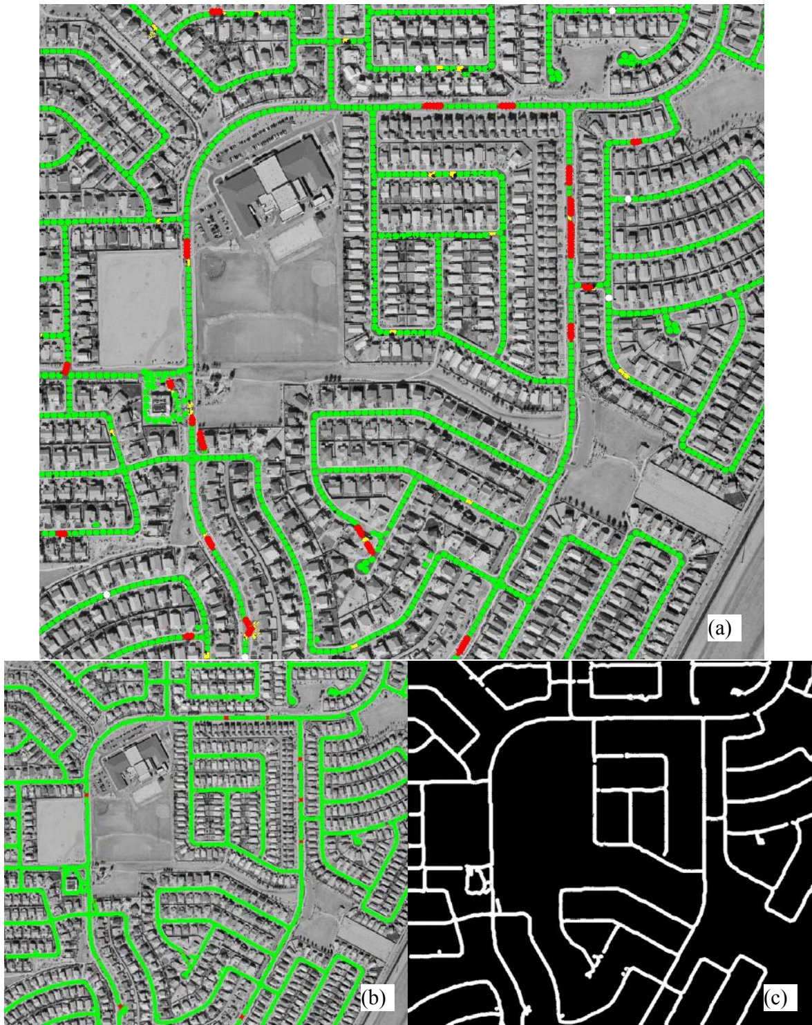
Figure 4.21 Roads in black and white aerial image detected by the RoadModeler
