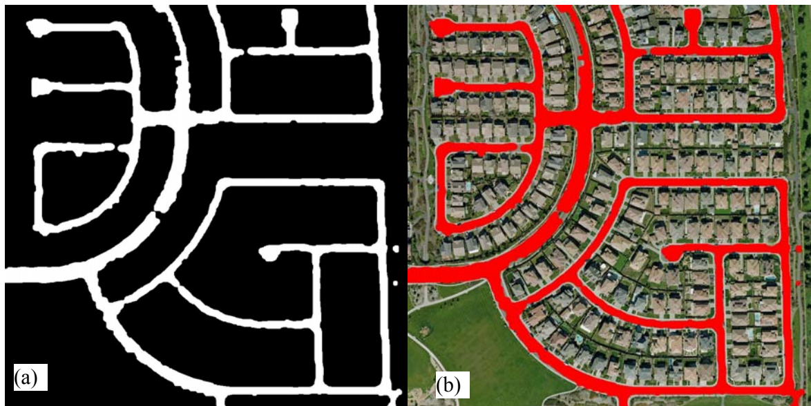
Figure 4.17 Morphologically filtered roads with few trees and overlaid on the image
