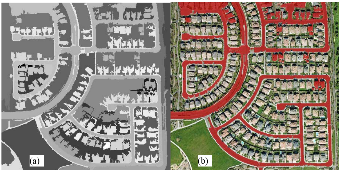
Figure 4.15 Roads with few trees detected by the object-oriented classification
