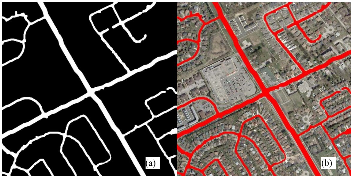
Figure 4.14 Morphologically filtered roads with parking lots and overlaid on the image
