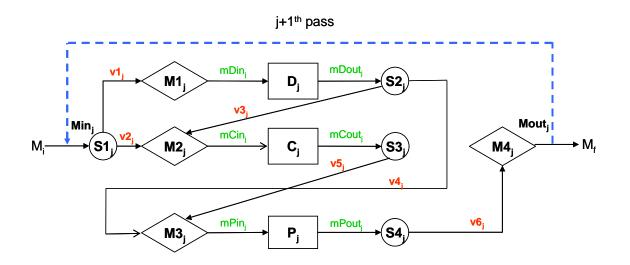
Figure 3.2. Three-alternative superstructure with the associated Boolean variables.
