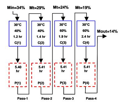
Figure 3.7 The optimal flowsheet of minimization of energy consumption with the ad hoc model from Case study1.
