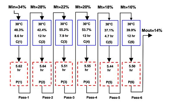
Figure 3.9. The optimal flowsheet of minimization of energy consumption from Case Study 2.
