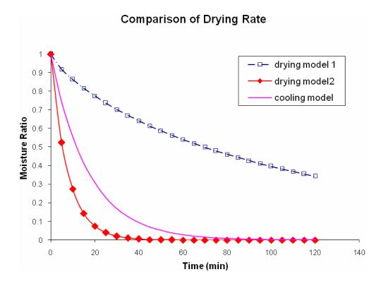
Figure 3.11. The comparison of drying rate from using different drying and cooling models.
