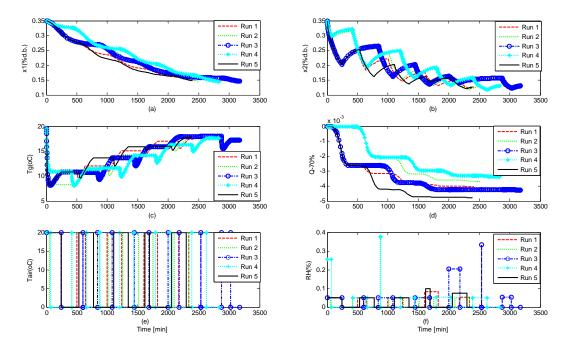
Figure 4.13. State and control profiles obtained from solving the synthesis problem with energy objective function from five runs.
