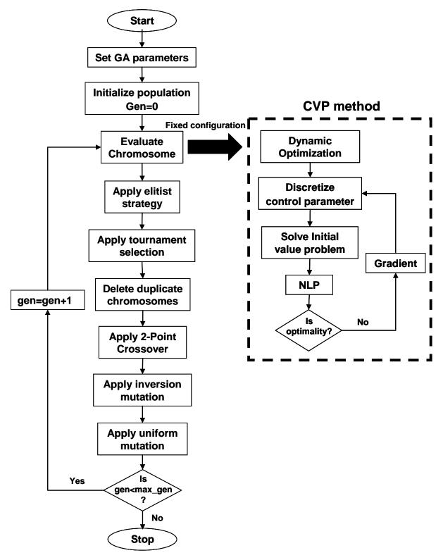
Figure 4.3. Algorithm structure of hybridization method.
