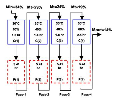
Figure 3.6 The optimal flowsheet of minimization of energy consumption with the GDP model from Case study1.
