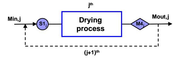
Figure 3.3. Input and output moisture content to a drying process in each pass.
