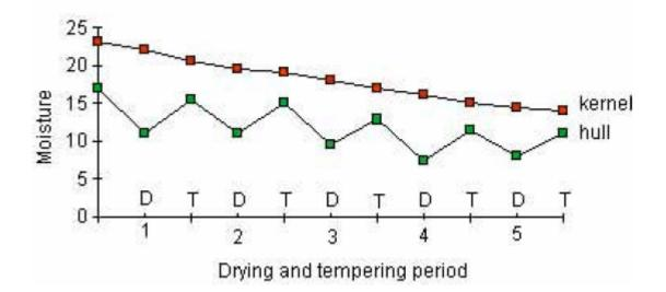
Figure 1.3 Moisture content of kernel and hull after each drying pass in five passes drying of rough rice (James, 1998).
