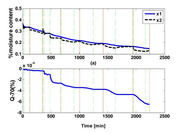
Figure 4.11. The state profiles of moisture contents and quality of rice grain from the best solution found from configuration "5 3 5 4 3 3 4 0".
