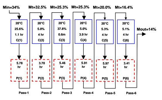
Figure 4.14. Optimum configuration of the synthesis problem with energy objective function using the theoretical model with 4 hr maximum cooling time allowed.
