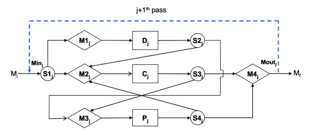
Figure 4.2. Superstructure of rice drying processes with 5 alternatives.
