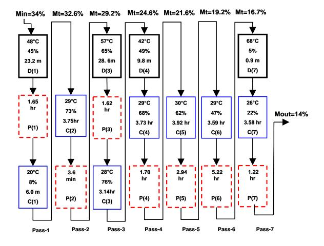
Figure 4.12. Optimum configuration of the synthesis problem with quality objective function using the theoretical model.
