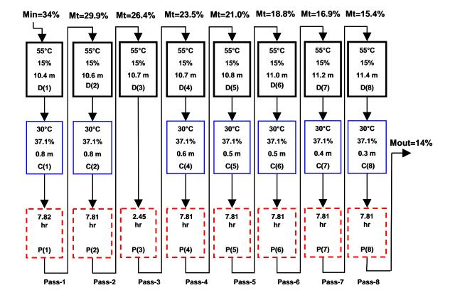
Figure 3.8 The optimal flowsheet of maximization of HRY from Case study 2.
