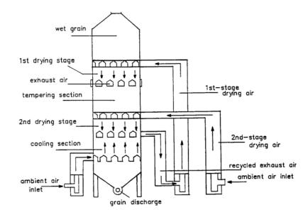
Figure 1.6. Two stage concurrent-flow dryer with counterflow cooler and tempering section (Brooker et al., 1992).
