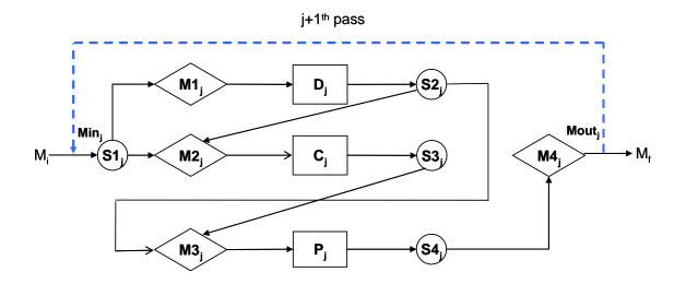
Figure 2.1. Three-alternative superstructure representation of synthesis of rice drying processes using empirical models.
