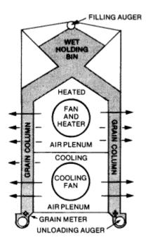
Figure 1.4. Conventional crossflow dryer with a drying and a cooling section (Brooker et al., 1992).
