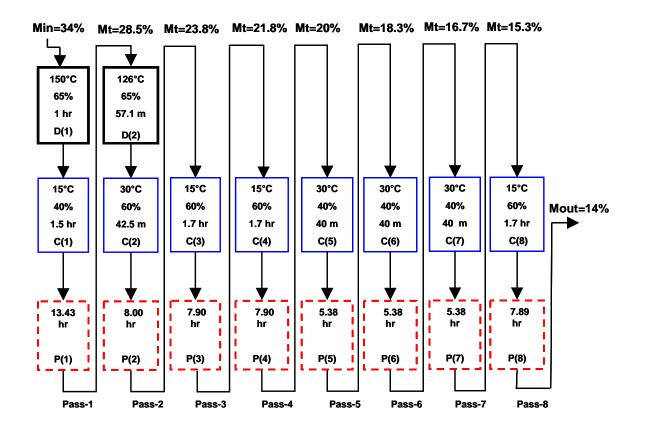
Figure 3.4 The optimal flowsheet of maximization of HRY with the GDP model from Case study 1.
