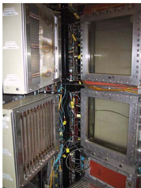
Figure 5.10 Miniplant-size Ni Foam plater (cca 1990)
