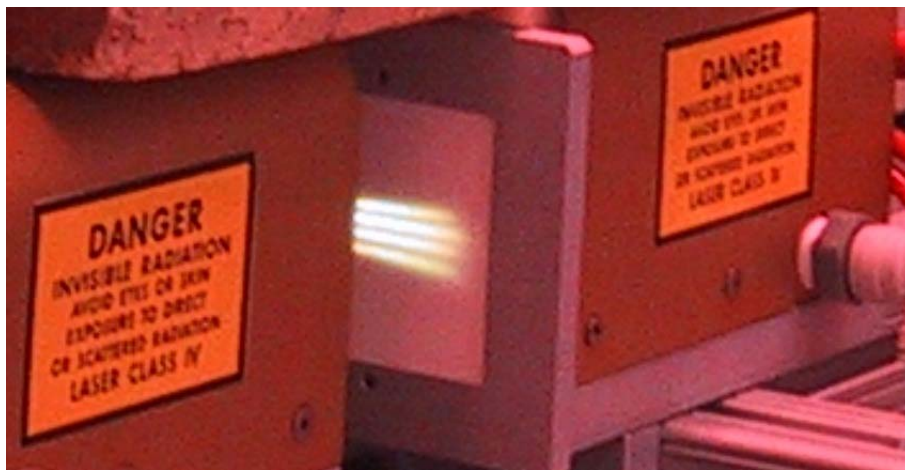
Figure 3.9 Part of the laser head beam with beam-shaping optics and homogenizer installed and imaged on the View-It ® ceramic plate
