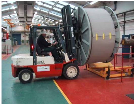
Figure 5.13 Large production spool of Ni foam being transported between sintering and slitting operations
