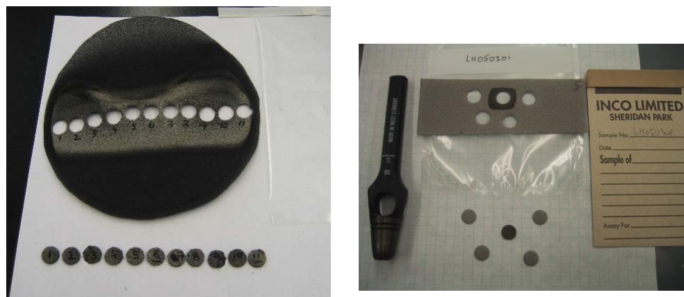
Figure 3.46 Deposit thickness measurement
