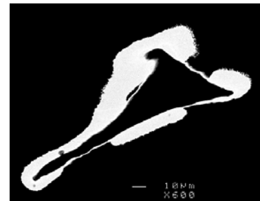
Figure 4.32 Cross-sections of the same sample, showing passivated areas
