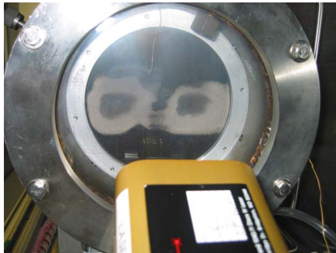
Figure 5.5 Flow patterns visible on Ni deposits prepared with 4x13 cm 2 sample opening
