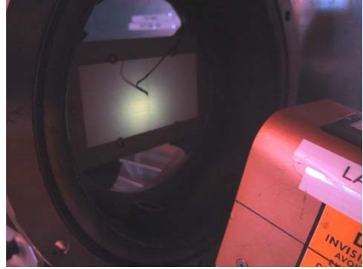
Figure 3.27 Beam shape with diffuser plate, lenses removed (North side)
