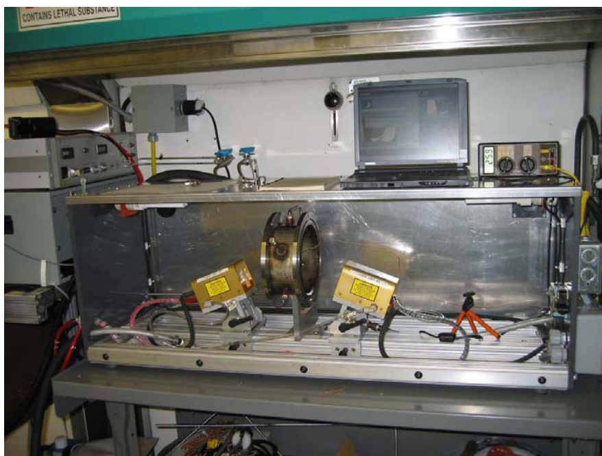
Figure 3.2 LCVD cylindrical reactor system shown shortly after assembly
