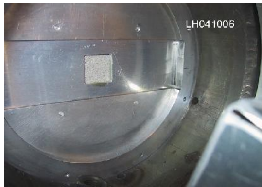
Figure 3.19 Improved 2x2 sample holder, uniform uni-directional flow
