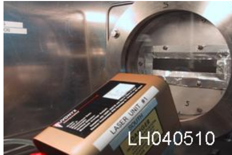
Figure 3.17 2x10 cm sample holder, improved flow uniformity
