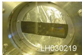
Figure 3.15 4x15 cm sample holder, non-uniform flow.
