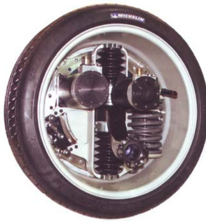
Fig. 1-8 Michelin active wheel with an active suspension system (Kendall, 2008).
