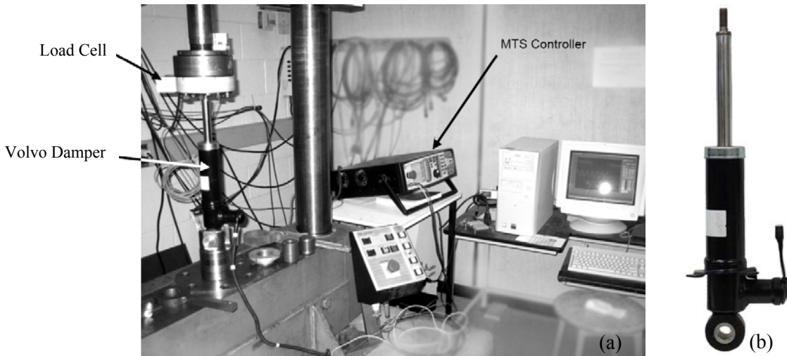
Fig. 2-1 (a) UW MTS shaker test setup (Vahid, 2006) and (b) Volvo S60 solenoid-valve damper.
