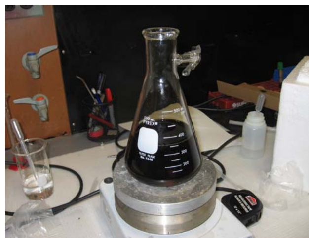
Figure 5-10. The Ag solutions which are prepared by the Lee procedures. The greenish yellow solution is prepared by citrate reduction procedures. This solution shows a strong SERS activity( Fig5-9). However, the second solution ( the colloid particles collapsed) shows no SERS activity.
