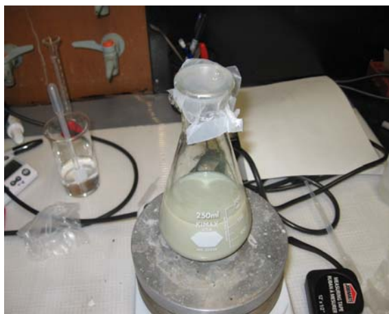
Figure 5-10. The Ag solutions which are prepared by the Lee procedures. The greenish yellow solution is prepared by citrate reduction procedures. This solution shows a strong SERS activity( Fig5-9). However, the second solution ( the colloid particles collapsed) shows no SERS activity.
