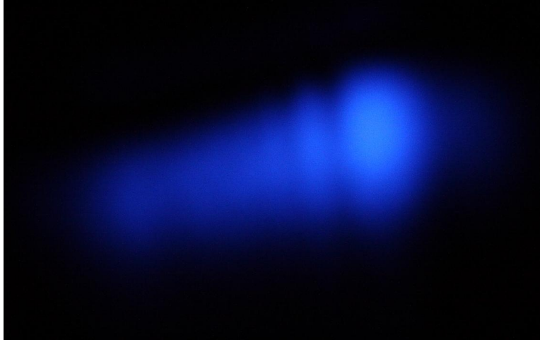
Figure 3.1: A photograph of the output of the BiBO frequency doubler. Note the sinc-like pattern in the horizontal direction. The beam was later optimized so that the brightest point was in the centre, and only this portion was used for my experiment with the rest removed using an aperture. Photograph courtesy Bill Rosgen
