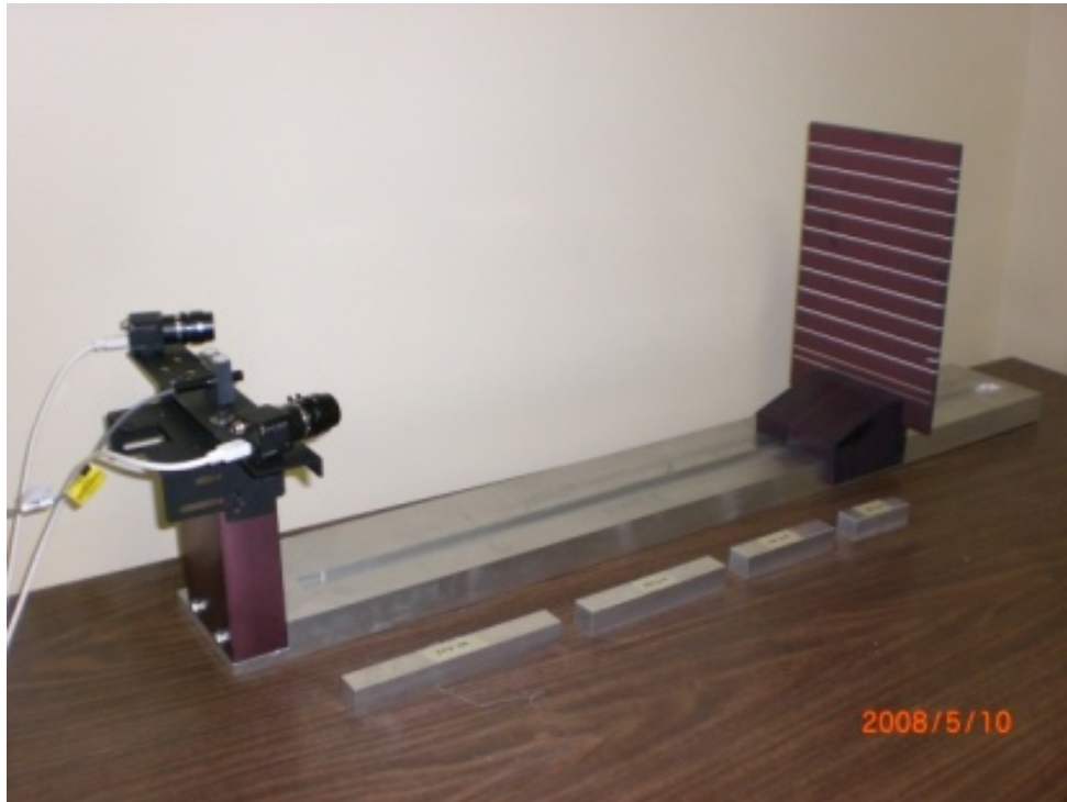
Fig. 4.6 Calibration jig with range-sensor and space bars.
