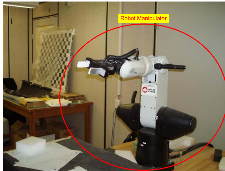
Fig. 3.3 Robot manipulator site of the robot teleoperation system. The robot manipulator has six joints for six degrees of freedom. There is a two-finger gripper at the end effector to perform object manipulation tasks. The fingers are closed to grab an object, and opened to release an object.
