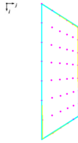
Fig. 4.13 Synthetic image of calibration points for one laser projection. There are 48 image blobs corresponding to 48 calibration points.
