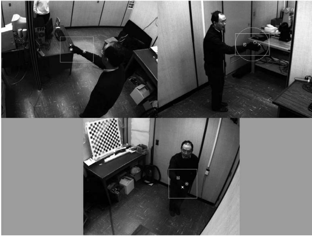
Fig. 3.5 Hand tracking with all markers visible in all cameras. The top-left image is captured from the left camera, top-right from the right camera, and bottom one from the mid camera. The big white rectangles in the images are the current search windows for markers. The large circle in the right image shows that the markers in this image are back-projected from the markers' true 3D coordinates in space. Back-projection takes place in the right image since the primary (left-mid) stereo camera pair is utilized in this frame; therefore, the right image is simply ignored in computing the 3D locations of the markers. The three markers are correctly matched and labeled. The markers marked by a square, circle, and cross are the wrist, thumb, and index-finger markers, respectively.
