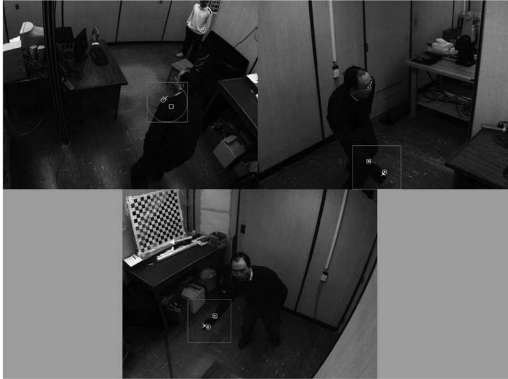
Fig. 3.6 Hand tracking with marker occlusion. Occlusion occurs in the left image and invalidates the primary camera pair. The mid-right camera pair is utilized instead. Back-projection takes place in the marker-missing image (left). The occlusion problem is hence solved by the proposed camera utilization scheme. This approach is also used when all the markers are totally occluded in an image.
