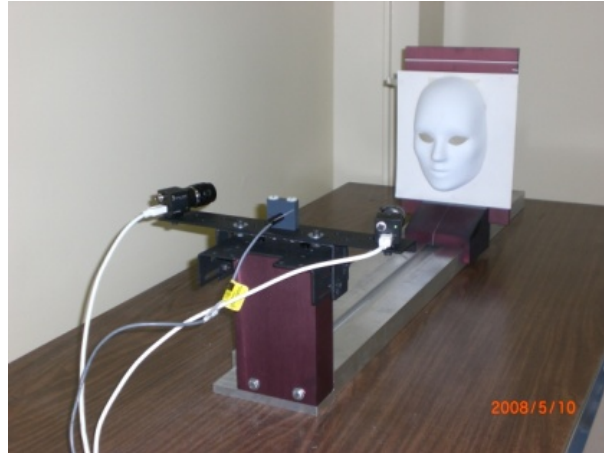
Fig. 4.8 Object placed in calibration volume. For surface-geometry measurement of an object, the object (here a human mask) must be placed within the calibration volume.
