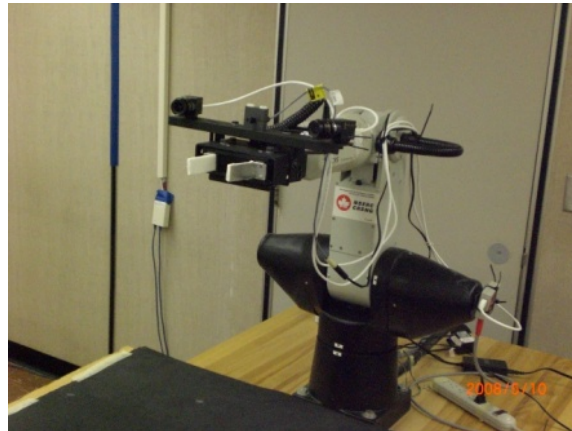
Fig. 4.1 Robot manipulator with range sensor mounted on the end effector.
