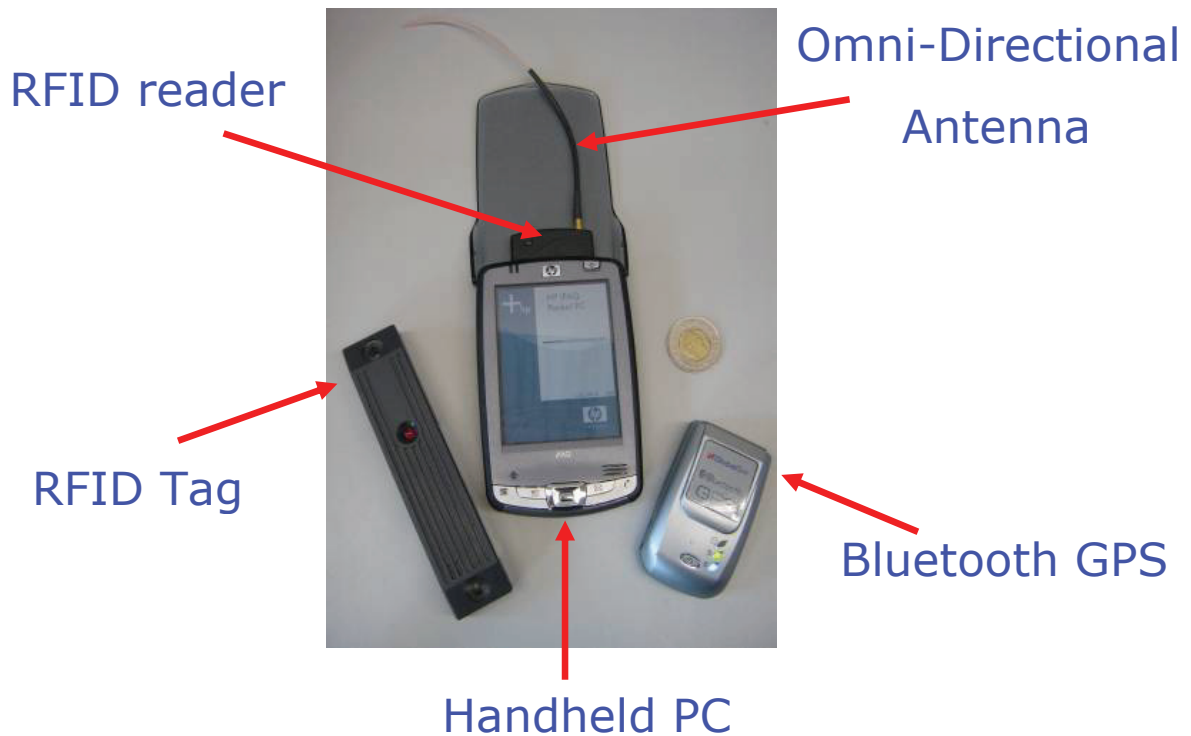
Figure 4.8: Components used in the automated materials tracking process
