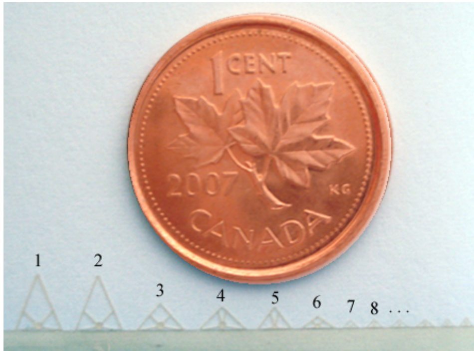
Figure 4.12: The fabricated SU-8 microgrippers of various sizes.
