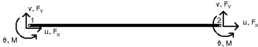
Figure L.3: Schematic of Beam Element
