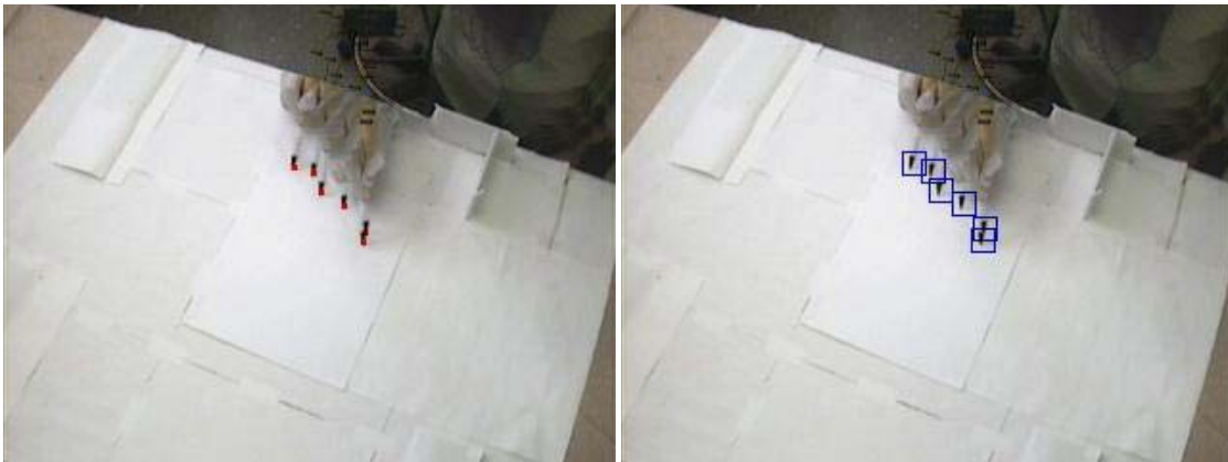
Figure 66 - Tool tip tracking by camera #3
