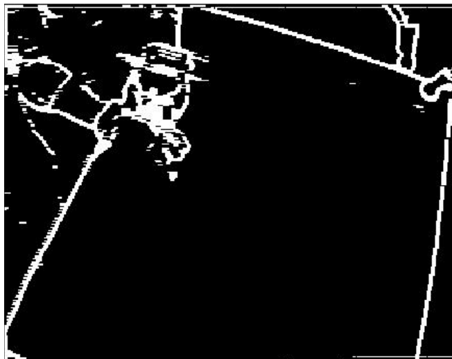
Figure 60 - The effect of opening morphologic operations followed by closing operation
