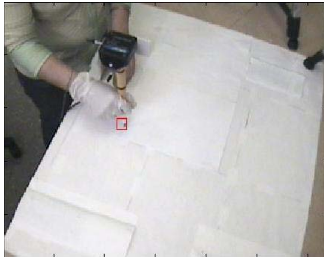
Figure 62 - Initial guess window mask for the position of tool tip
